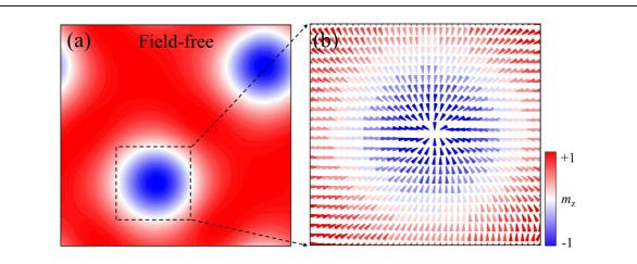
FIG. 4. (a) Atomistic spin model simulated spin configurations for a curved MnSe<sub>2</sub> with size of curvature c of 31.6%, (b) zoom in of an isolated skyrmion profile.
