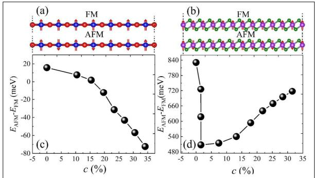
FIG. 6. (a) and (b) are FM and AFM spin configurations of  $CrBr_2$  and  $MnSe_2$ . (c) and (d) are the energy differences between AFM and FM for  $CrBr_2$  and  $MnSe_2$  under different size of curvature c, respectively.
