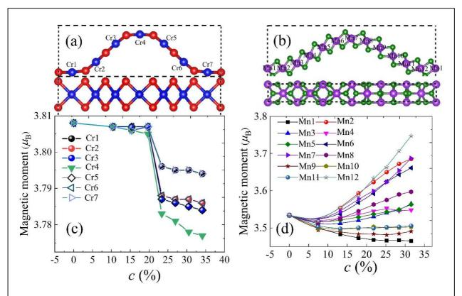
FIG. 7. (a) and (b) show curved 1D  $CrBr_2$  and 2D  $MnSe_2$  structures, respectively. (c) and (d) represent the absolute value of magnetic moment per Cr and Mn atom as c increases, respectively.
