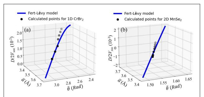
FIG. 9. Plotted theoretical curve and calculated results by using Fert-Lévy model (Eq. (2)). (a) and (b) indicate that the  $D/2V_{\rm soc}$  as a function of average bond angle  $\bar{\theta}$  and average bond length  $\bar{a}$  in 1D CrBr<sub>2</sub> and 2D MnSe<sub>2</sub>, respectively.
