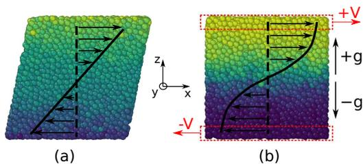
FIG. 1. The two flow configurations studied in this Letter: (a) homogeneous shear flow and (b) concave flow. Cell height is  $20d$ . The lighter yellow corresponds to the largest velocity to the right, and the darker blue corresponds to the largest velocity to the left.
