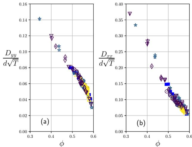
FIG. 4. (a) Transverse ( $D_{yy}$ ) and (b) streamwise ( $D_{xx}$ ) self-diffusivities, as determined from numerical simulations, scaled by the square root of granular temperature, versus solid volume fraction. The symbols have the same significance as in Fig. 3.
