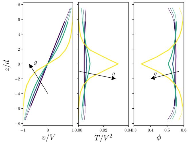
FIG. 2. Average flow profiles in the concave flow, for a global value of solid fraction of  $\phi \approx 0.55$  and different values of acceleration  $g$  (respectively  $g = 10^{-7}, 10^{-6}, 2 \times 10^{-6}, 3 \times 10^{-6} \frac{dk_B}{m}$  when going from dark blue to yellow): (a) streamwise velocity, (b) granular temperature, (c) solid fraction. The part of the profiles in bold corresponds to data points which were used for the self-diffusion analysis.
