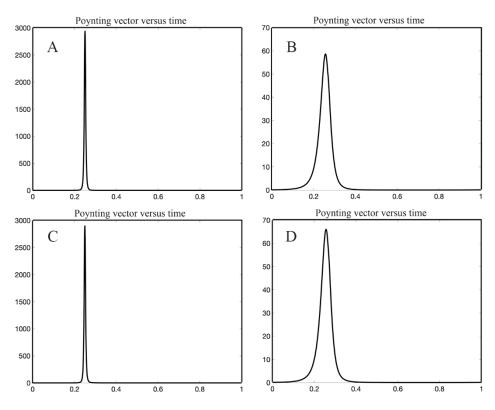
Fig. 1. Flow of energy at the exit to a grating as a function of time normalised to unit incident flux. The abscissa covers one time period of the grating. In each case  $\Omega = g = 1.0$ ,  $\omega = 0.3$ , d = 10, otherwise:
