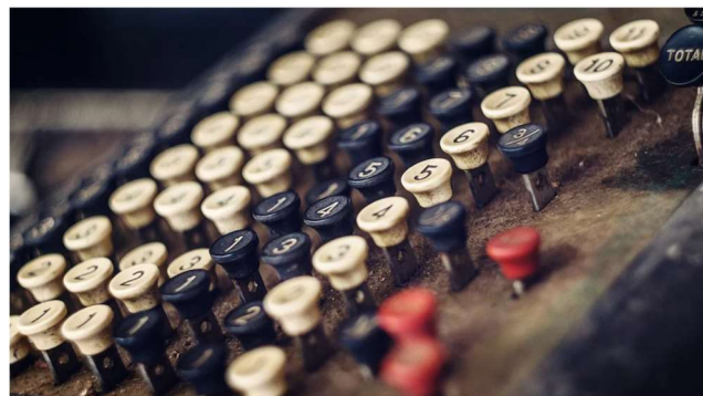
Figure 2. | A mechanical cash register computes at the expense of spring stored power drawn from the user hitting keys and pulling levers. It dissipates a fair amount of it in wear and friction.
