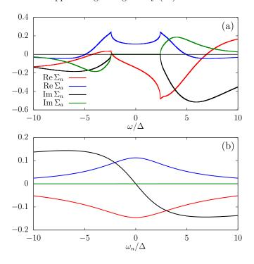
FIG. 1. Normal and anomalous components of the self-energy calculated using the second-order perturbation theory for  $U = 4\Delta$ ,  $\Gamma = 2\Delta$ ,  $\varepsilon = 2\Delta$ ,  $\varphi = 0$  and T = 0 along the real (a) and imaginary frequency axis (b).
