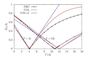
FIG. 7. ABS energy  $E_0/\Delta$  as a function of the interaction strength U for the same parameters as in Fig. 2:  $\varepsilon = 0$ ,  $\varphi = 0$ and two values of the tunneling rate  $\Gamma = \Delta$  and  $\Gamma = 2\Delta$ , calculated using GAL including the band correction C (solid red), without the correction (dashed blue) and NRG (black). The effect of the band correction is stronger at larger values of  $E_0$  and vanishes exactly at the transition point ( $E_0 = 0$ ).
