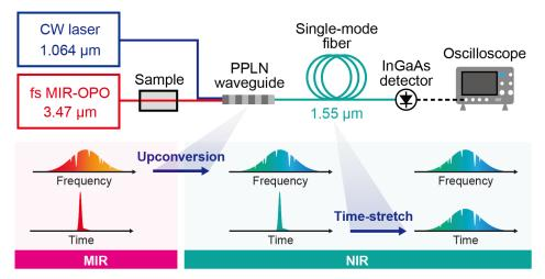
Figure 2: Schematic of upconversion TSIR (UC-TSIR). MIR-OPO: mid-infrared optical parametric oscillator, PPLN: periodically-poled lithium niobate.
