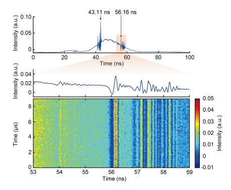
**Supplementary Figure 7:** Wavenumber instability of TSIR spectroscopy. The upper and middle panels show the averaged TSIR spectrum measured at 10 Mspectra/s with the 30-km DCF and the enlarged view of the spectrum in the time frame of 53-59 ns, respectively. The lower panel represents the temporal variation of single-shot TSIR spectra in the time frame of 53-59 ns sequentially measured at 10 Mspectra/s.
