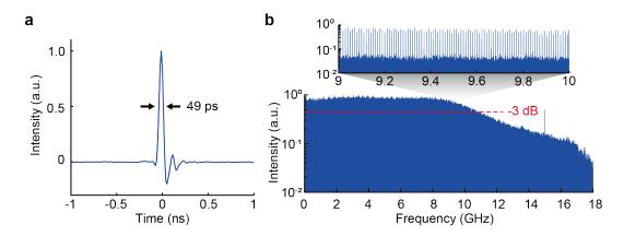
**Supplementary Figure 5:** Characterization of the InGaAs photodetector used in our experiment. **a** An impulse response of the detector. The FWHM width is 49 ps. **b** Frequency response of the detector. The -3dB bandwidth is 11 GHz.
