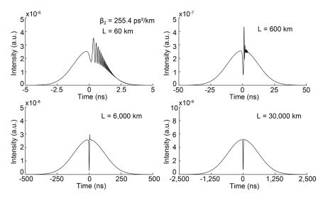
Supplementary Figure 6: TSIR waveforms calculated with various amounts of dispersion. We calculate a 1-cm<sup>-1</sup>-width gaussian-shape spectrum with a 0.01-cm<sup>-1</sup>-width absorption line and temporally stretch it using fibers with a GVD of 255.4 ps<sup>2</sup>/km at four different lengths (60, 600, 6000, and 30000 km).  $\beta_2$ : GVD, *L*: fiber length.
