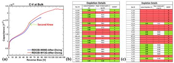
Figure 8: (a) Bulk C-V plot of RD53B sensors after dicing, and C-V summary after dicing: (b) W09 and (c) W13.
