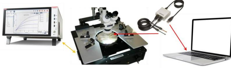
**Figure 3:** UniTN sensor QC probing setup.
