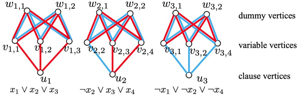
■ **Figure 4** An example of reducing a 3-CNF formula to a graph in EXISTS-PMVC-DD.
