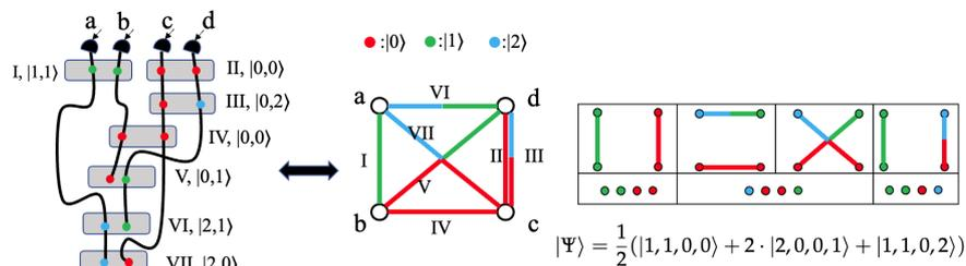
■ **Figure 3** Left: a quantum optical circuit corresponding to the graph in Figure 1. Each crystal (shaded box) correspond to an edge in graph. Each optical path is converted into a vertex in graph. The modes of photons translate to edge colors. Right: all PMs in the graph reflect the quantum state of the optical circuit as a superposition of coincidences. [23]
