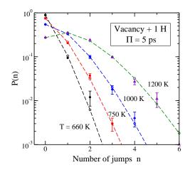
FIG. 9: Probability distribution for the number of H jumps in a time window  $\Pi = 5$  ps. Solid symbols represent results derived from MD simulations at T = 660 (circles), 750 (squares), 1000 (diamonds), and 1200 K (triangles). Open circles joined with dashed lines indicate the expected Poisson distribution corresponding to the same time window  $\Pi$ . Error bars of the simulation results, when not shown, are in the order or less than the symbol size.
