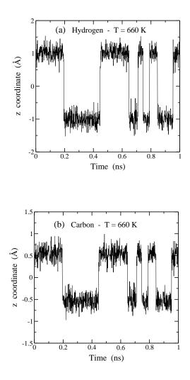
FIG. 6: Coordinate z of (a) hydrogen and (b) carbon along a MD simulation run at 660 K. Both atoms form a C–H bond. The data shown include  $2 \times 10^6$  MD steps, corresponding to a time interval of 1 ns.
