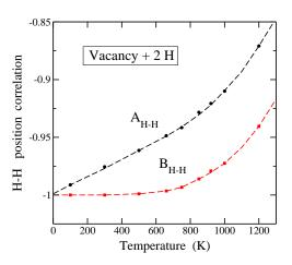
FIG. 11: Temperature dependence of the correlation functions  $A_{\rm H-H}$  and  $B_{\rm H-H}$  for the z coordinate of both H atoms close to a carbon vacancy. These functions are defined in Eqs. (5) and (6). Symbols are data points derived from MD simulations. Dashed lines are guides to the eye.
