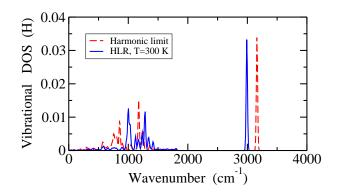
FIG. 2: Vibrational density-of-states for hydrogen in defective graphene. The dashed line represents the DOS obtained from diagonalization of the dynamical matrix (harmonic approximation), whereas the solid line represents the DOS derived from HLR calculations at 300 K.
