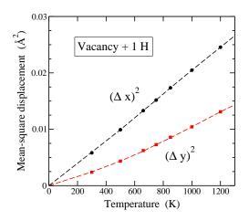
FIG. 5: Mean-square displacement of H along the x and y directions. Symbols indicate results of MD simulations at several temperatures: circles for  $(\Delta x)^2$  and squares for  $(\Delta y)^2$ . Dashed lines are guides to the eye. Error bars are less than the symbol size.
