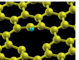
FIG. 1: Ball-and-stick image of an atomic configuration taken from a MD simulation of H close to a carbon vacancy in graphene. Yellow balls represent C atoms, whereas the small blue sphere represents the hydrogen atom. The simulation was carried out at T = 300 K.
