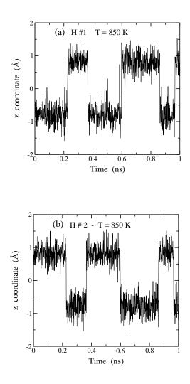
FIG. 10: Coordinate  $z_{\rm H}$  of both H atoms close to a C vacancy along a MD simulation run at T = 850 K. The data shown in (a) and (b) correspond to H #1 and H #2 in a time interval of 1 ns (2 × 10<sup>6</sup> MD steps).
