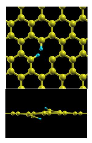
FIG. 3: Top (upper) and side (lower) views of the minimumenergy configuration for two H atoms at a carbon vacancy in graphene. Yellow large balls and small blue spheres represent C and H atoms, respectively.
