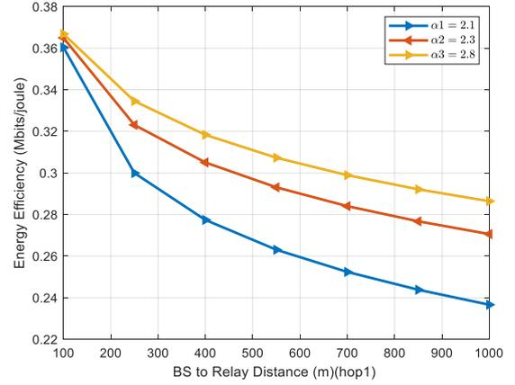
Figure 2: Energy efficiency performance versus distance between the active BS and relay with different path loss exponents and bandwidths.
