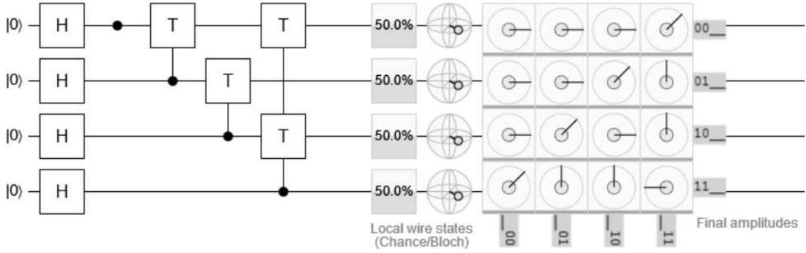
Figure 3. Example 2. Circuit for  $|M_1\rangle$  with  $T$  gates
