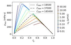
Figure 4: Apparent viscosity  $\mu_{app}$  as a function of  $u_{g}$  and  $f_{g}$ , all using LE foam, for the non-Newtonian foam model. The dashed and dotted lines represent Newtonian total apparent viscosity with a given  $C_{MRF}$ .
