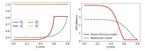
Figure 2: Wave profiles in the non-Newtonian (filled lines) and Newtonian (dashed lines) models using  $K_c = 200 \text{ s}^{-1}$  in Scenario 2. Left:  $\tilde{S}_w(\xi)$  and  $\tilde{n}_D(\xi)$ . Right: pressure gradient obtained using the formulas from Section 2.
