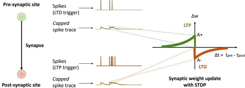
Figure 2: Online implementation principle of STDP using local pre- and post-synaptic capped spike traces which provide an online estimate of the time since the last spike. For example, at the moment of post-synaptic spike, potentiation is induced with a weight change that is proportional to the value of the pre-synaptic spike trace, and the post-synaptic spike trace is updated with a jump to  $A_-$ .
