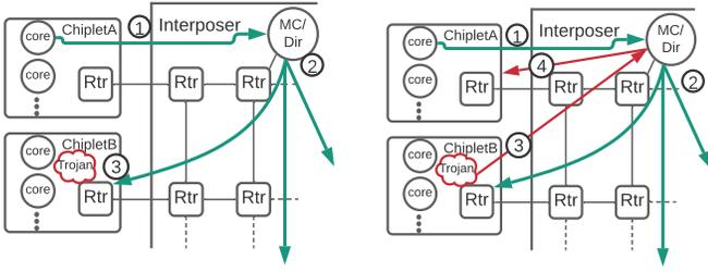
(a) **Passive Reading:** Trojan passively observes write traffic for other chiplets. (1) Misses from Chiplet A cause (2) broadcast invalidations to all chiplets; (3) Trojan snoops invalidation addresses.
