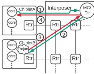
(c) **Modifying:** Trojan modifies a message to achieve incoherent state. (1) Chiplet A sends GETX to directory; (2) directory forwards request to Trojan's core which has line in 'E' state. Trojan blocks GETX and (3) replies with GETX to requestor, (4) invalidating Chiplet A's cache entry, leaving attacker in control of another cache's contents.
