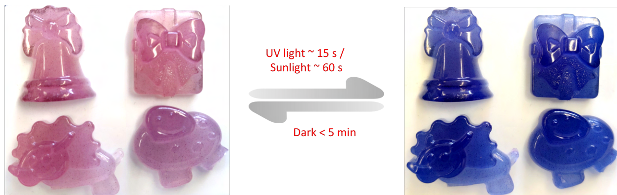
Fig. S48. Photographs of various shaped sculptures fabricated from 0.5 wt.% loading of 8NSP@ZIF-71(20) in PDMS polymer matrix. The photographs show the visual color switching upon exposure to 365 nm UV light or sunlight.
