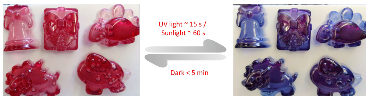
Fig. S49. Photographs of various shaped sculptures fabricated from 0.5 wt.% loading of 8NSP@ZIF-71(20) in PS polymer matrix. The photographs show the visual color switching upon exposure to 365 nm UV light or sunlight.
