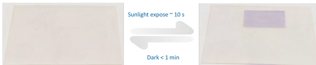
Fig. S64. Using inkjet printing technology, NSP@ZIF-71(20) was printed as two layers on an indium tin oxide (ITO)-coated glass substrate to demonstrate the color-changing phenomenon in the presence of sunlight. A DMF solvent was used to prepare the sample. The printed film sample was invisible to the naked eye under ambient room conditions but became visible (against a white background) after exposure to sunlight for ~ 10 s.
