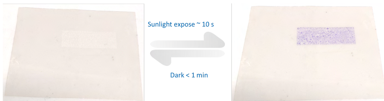
Fig. S65. Using inkjet printing technology, NSP@ZIF-71(20) was printed as two successive layers on an ITO-coated flexible acetate sheet to demonstrate the color-changing phenomenon in the presence of natural sunlight. A DMF solvent was used to prepare the sample. Initially, the printed film sample was invisible to the naked eye under ambient room conditions, but it became visible (against a white background) after exposure to sunlight for ~ 10 s.
