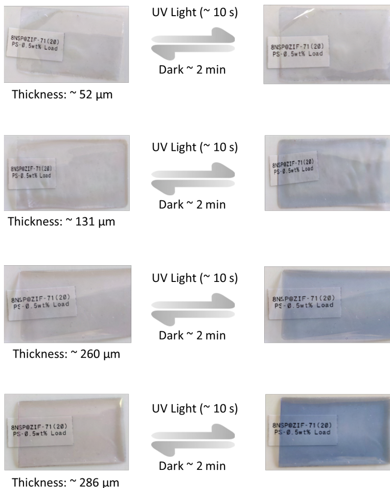
Fig. S40. Photographs of different thickness of PS film with 0.5 wt.% loading of 8NSP@ZIF-71(20). The optically transparent PS film changes color after being exposed to 365 nm (6W) UV light for 10 seconds, returning to its original color in less than 5 minutes. The color switching phenomenon becomes more prominent with increasing thickness of the films where loading of the filler was fixed for each case.
