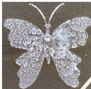
Fig. S61. Using inkjet printing technology, NSP@ZIF-71(20) was printed to form two layers on a glass substrate to demonstrate the color-changing phenomenon in the presence of various ambient lighting conditions. An IPA solvent was used to prepare the sample.
