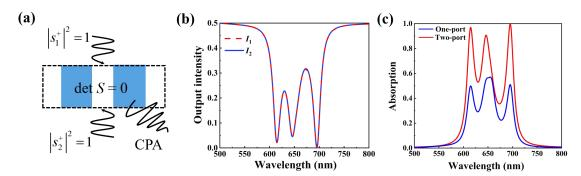
FIG. 6. (a) Schematic diagram of coherent perfect absorption. (b) The output intensities  $I_1$  and  $I_2$  of the system under two-port source excitation. (c) The absorption spectra of the system under one-port and two-port source excitation, respectively.
