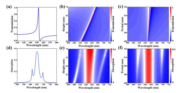
FIG. 3. (a) The transmission spectrum of the quasi-BIC with g = 127 nm. Transmission spectra of the quasi-BIC with respect to (b) height and (c) period. (d) Absorption spectrum of hybrid mode with gap g = 127 nm and height h = 61 nm. Absorption spectra of hybrid modes at different (e) height and (f) period.
