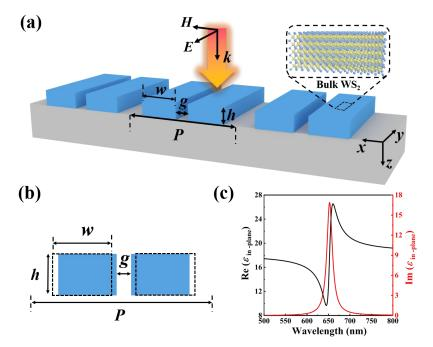
FIG. 1. (a) Schematic diagram of dimerized gratings composed of bulk WS<sub>2</sub>. (b) The *xz* cross-sectional of unit cell of the structure, with the dashed boxes corresponding to the case g = 145 nm. (c) Real and imaginary parts of the in-plane dielectric function ( $\varepsilon_{in-plane}$ ) of bulk WS<sub>2</sub>.
