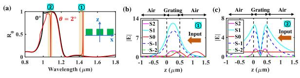
**Fig. 4.** Resonance spectra and leaky-mode profiles under a-GMR. (a)  $R_0$  spectra at  $\theta$ =0° and  $\theta$ =2° of the model 1D optical lattice {Λ=1 μm, F=0.5, H=0.5 μm, n=2} at a crosscut of Figs. 4(d) and 4(e) at Λ=1 μm. For a-GMR reflectance peak and null at ① and ②, the corresponding leaky-mode profiles are presented in (b) and (c).
