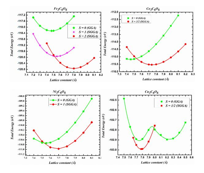
*Figure 1:* Total energy versus lattice constant for the free-standing  $TM_3C_6O_6$  structures calculated with the SGGA.
