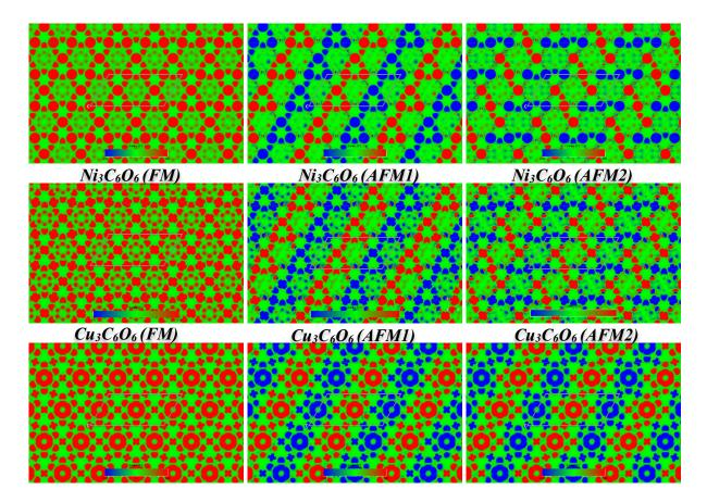
**Figure 3:** Cut plane of the spin density contribution with isovalue of  $\pm 0.02$  of  $TM_3C_6O_6$ . The spin surface is shown in the x-y plane like the atomic structure. The ferromagnetic arrangement and two different antiferromagnetic arrangements are shown and the results are obtained with SGGA+U.
