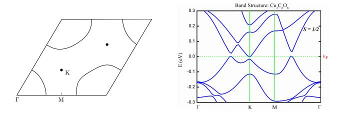
**Figure 7:** Fermi surface (a, left) without SO coupling consisting of a circle around  $\Gamma$  and two isolated points in the Brillouin zone, and band-structure (b, right) including SO coupling which opens a gap for the Cu<sub>3</sub>C<sub>6</sub>O<sub>6</sub> network calculated with the PAW-SGGA+U method.
