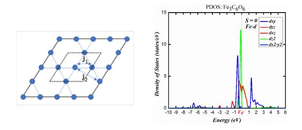
**Figure 4:** Schematic representation of the kagome lattice with the exchange couplings  $J_1$  and  $J_2$  (a, left) and partial, orbital resolved 3d DOS for  $Fe_3C_6O_6$  in GGA (no spin-polarized and without U correction) to illustrate the ligand field splitting (b, right).
