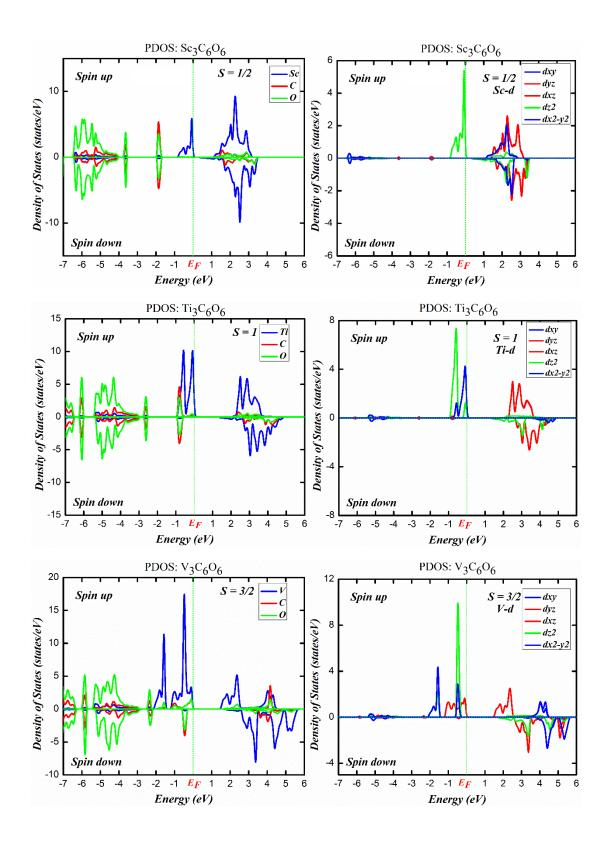
**Figure 6a:** Projected DOS of the atoms (TM, C and O) and d orbitals on the TM atoms in the 2D  $TM_3C_6O_6$  materials with the PAW-SGGA+U method for the TMs Sc, Ti, and V.
