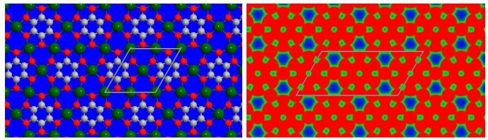
*Figure 2:* Geometrical structure and charge density of a free-standing structure of TM atoms and  $C_6O_6$  molecule (C: grey, O: red, and TM: Green).
