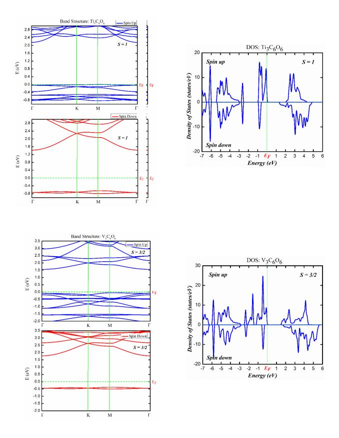
**Figure 5a:** Band-structures and total DOS of the 2D transition-metal (TM) -  $C_6O_6$  networks with the PAW-SGGA+U method, when TM is Sc, Ti, and V, respectively.
