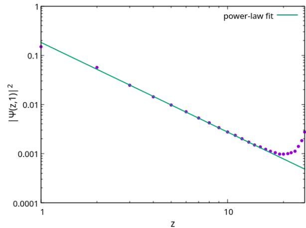
FIG. 5. Log-log plot of eigenstate's probability projected onto sublattice  $\alpha = 1$ , for the state with energy closest to  $E = 0$ , for  $L = 26$  and  $W = 0.5$ . In this example, the probability decays approximately as  $z^{-1.8}$  into the bulk.
