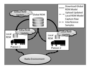
Fig. 3. Two-Layer REM architecture with FL cycle marked.
