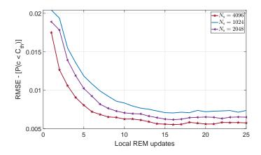
Fig. 8. RMSE computed between the outage probability estimated with the use of updated Local REM and the baseline model, for k = 5. Results are averaged over 50 simulations.
