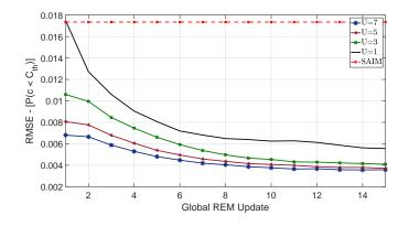
Fig. 10. RMSE computed between the outage probability estimated with the use of Global REM and the baseline model, for  $N_{\rm s} = 4096$ , k = 5, and the varying number of platoons U. Additionally, the results of the SAIM scheme are included. Results are averaged over 50 simulations.
