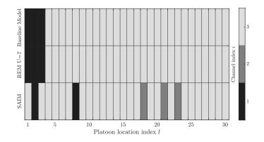
Fig. 11. Index *i* of channel offering the lowest outage probability in the consecutive platoon locations  $\mathbf{x}_l$  computed on the basis of baseline, Global REM, and Spectrum Sensing interference model.
