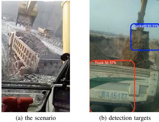
Fig. 5: A Virtual Excavator Supervisor with Smart Helmet
