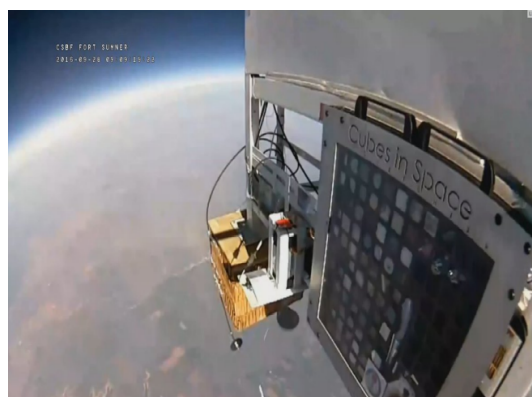
Figure 4.3: The Cubes in Space™ carrier on a NASA scientific balloon at float including about 100 individual experiments from grade 6 to 12 student teams.
