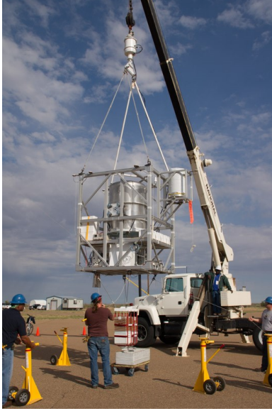
Figure 2.10: The GRAPE instrument prior to its launch from Fort Sumner in 2011. GRAPE aims to measure polarization of gamma-ray bursts.
