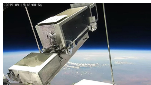
Figure 2.30: The BITSE coronagraph is pointed toward the Sun during its September 2019 flight.
