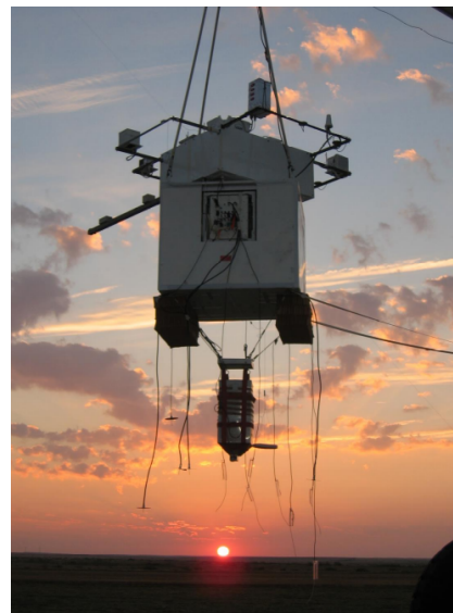
Figure 4.1: The High Altitude Student Platform (HASP) which carries multiple student development payloads to the edge of space was highlighted in the 2018 COSTEM report as an exemplary example of transdisciplinary learning.
