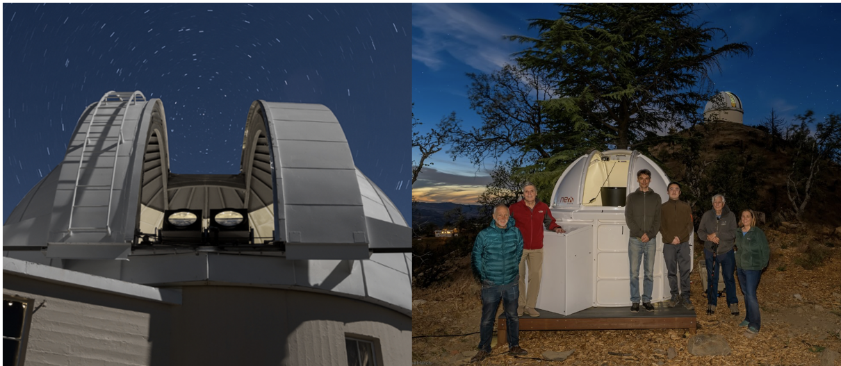
Figure 1. LEFT: Two PANOSSETI telescopes were deployed inside the Astrograph dome at Lick Observatory. RIGHT: The deployment of a third telescope at a distance of 677 m from the Astrograph confirmed the benefit of using a long baseline to identify and characterize transient phenomena (Left and right photos: courtesy Laurie Hatch Photography).
