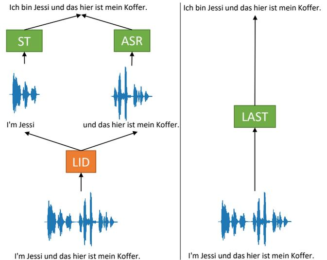
**Fig. 1.** Illustration of the information flow. Left: Baseline: Language identification (LID) followed by either the speech translation (ST) or automatic speech recognition (ASR) model. Right: Our LAST approach. For the green boxes, we use a transformer based encoder-decoder model. The transcripts in the middle and at the bottom are only shown for illustration purposes (the models don't have access to it).
