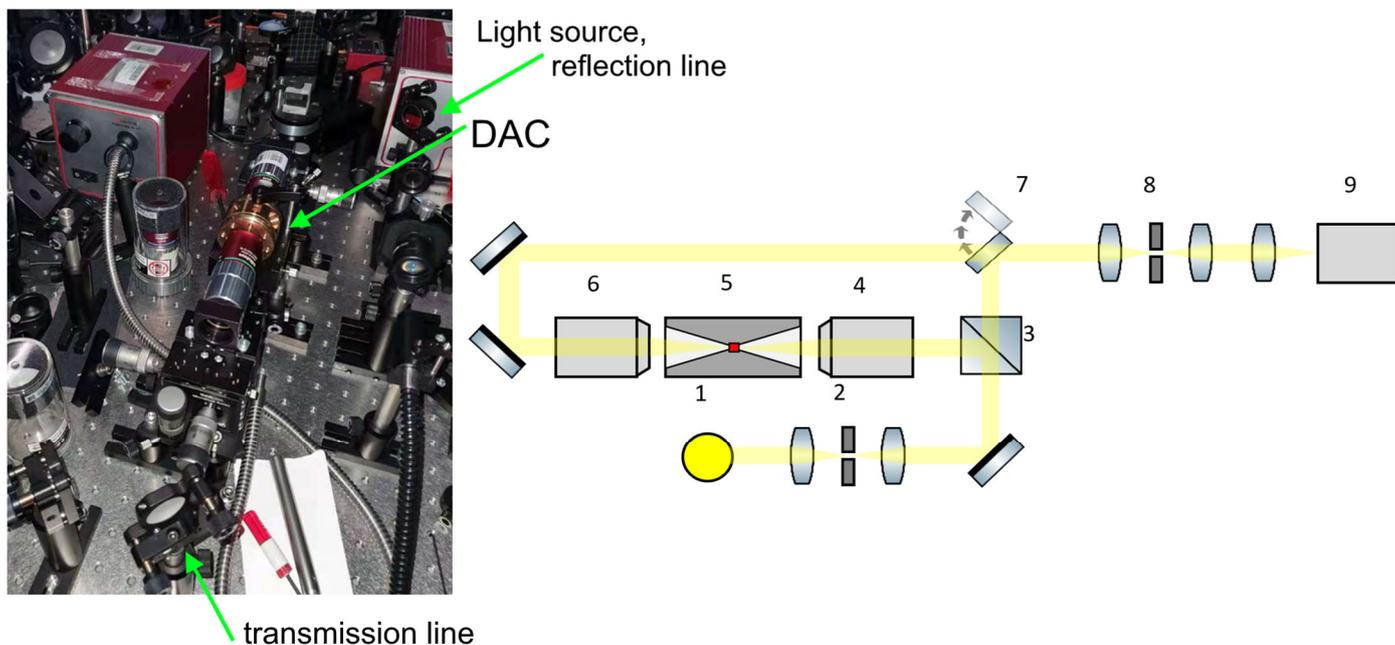
**Figure S13.** Optical scheme for transmission and reflection studying of samples in diamond anvil cells. 1 - Thorlabs OSL2B/OSL2BIR light source, 2 - a pinhole with diameter 50 $\mu$ m, 3 - beam splitter BS013, 4 and 6 - Mitutoyo plan apo NIR 20x infinity corrected objectives, 5 - the diamond anvil sample, 7 - flip mirror, 8 - a pinhole-type spatial filter and 9 - spectrometer with CCD camera: Action SpectraPro SP-2750 and ProEM HS.
