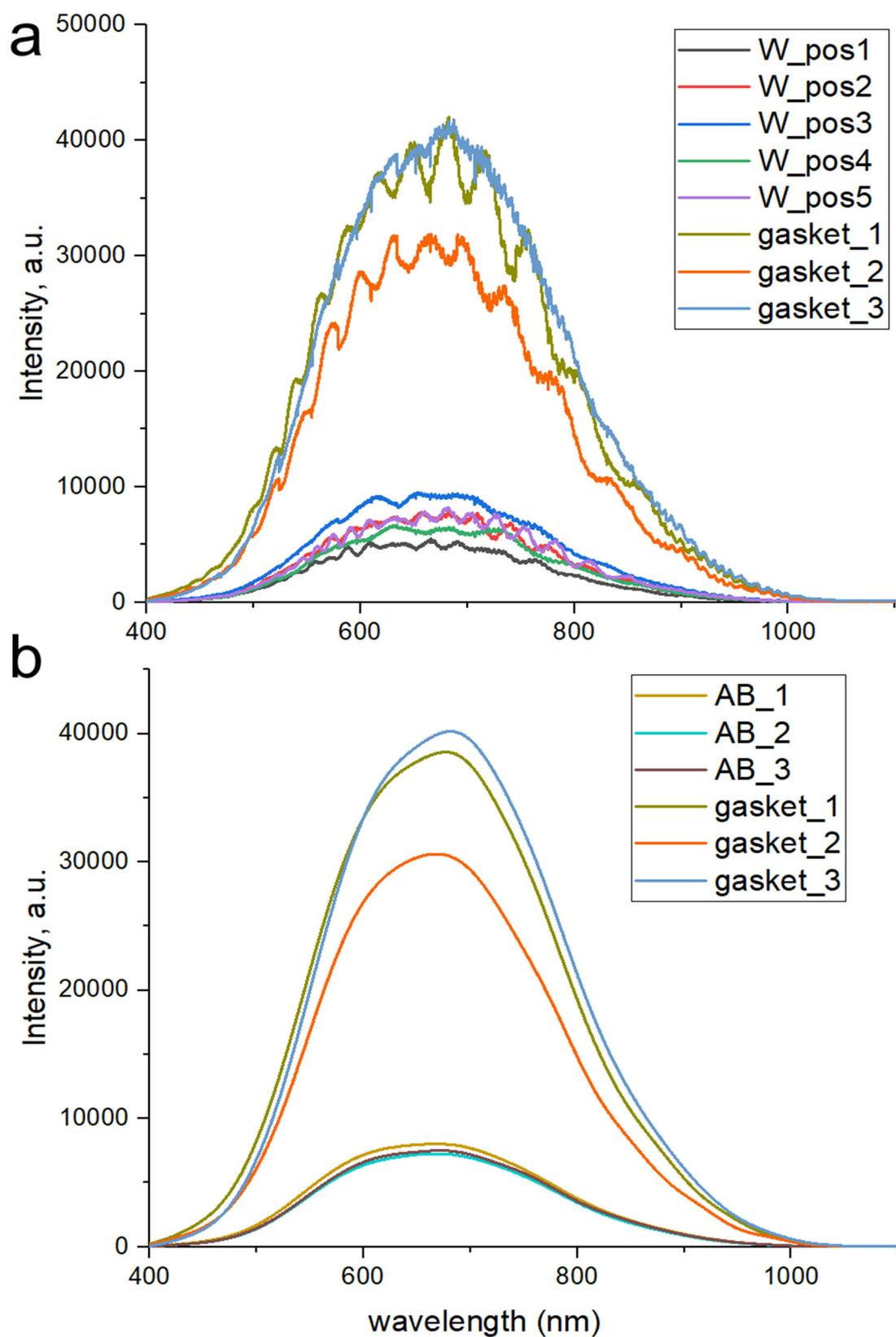
**Figure S21.** Reflectance spectra of the calibration DAC with the tungsten sample (W) in the ammonia borane medium (AB) and a rhenium gasket: (a) raw  $I(\lambda)$  data, (b) Fourier-filtered spectra.
