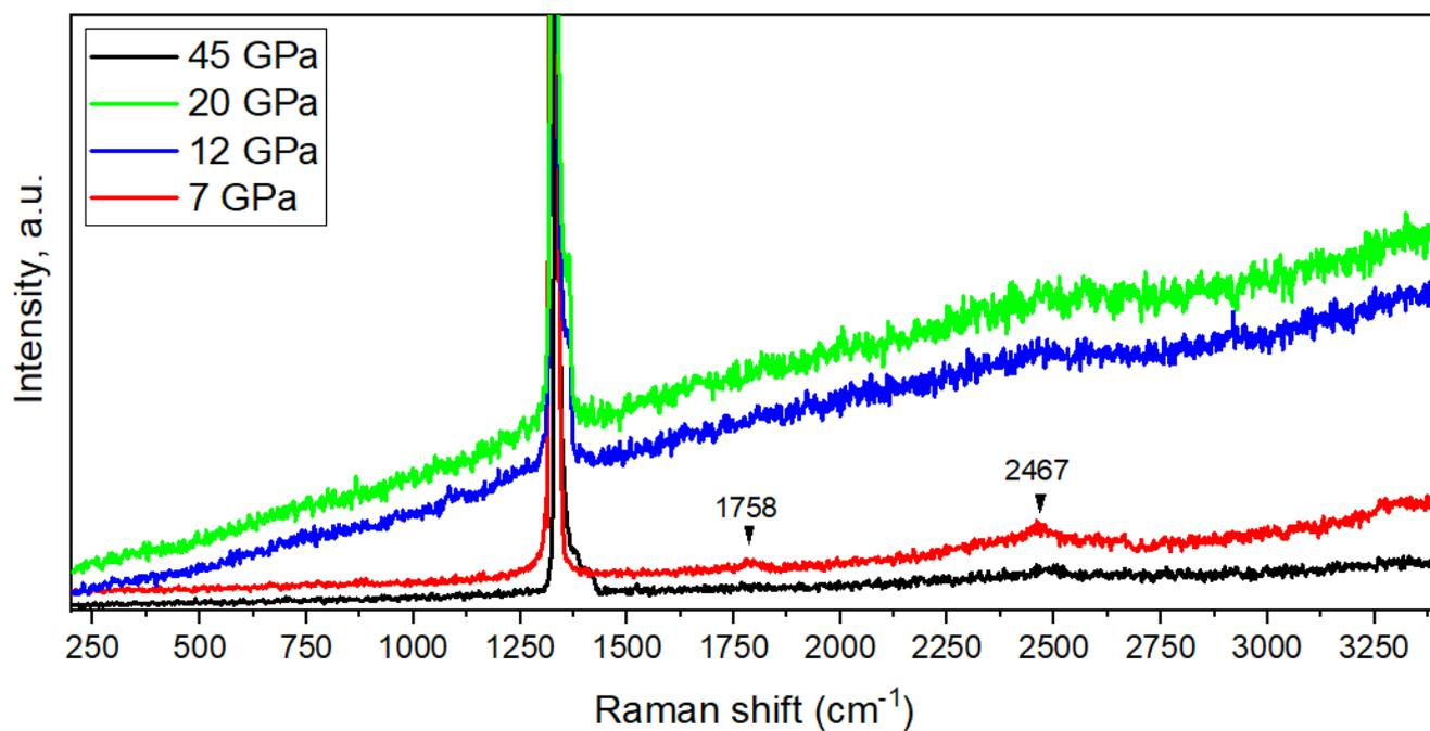
**Figure S11.** Raman spectra of the  $\text{TcH}_x$  samples taken at different pressures in the range of 250–3250  $\text{cm}^{-1}$ . There are weak signals (1758, 2467  $\text{cm}^{-1}$ ) from products of decomposition of ammonia borane (AB) and from AB itself.
