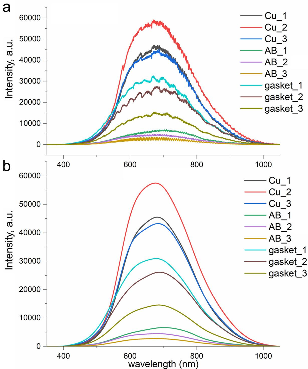
**Figure S22.** Reflectance spectra of the calibration DAC with the copper sample (Cu) in the ammonia borane medium (AB) and a rhenium gasket: (a) raw  $I(\lambda)$  data, (b) Fourier-filtered spectra.
