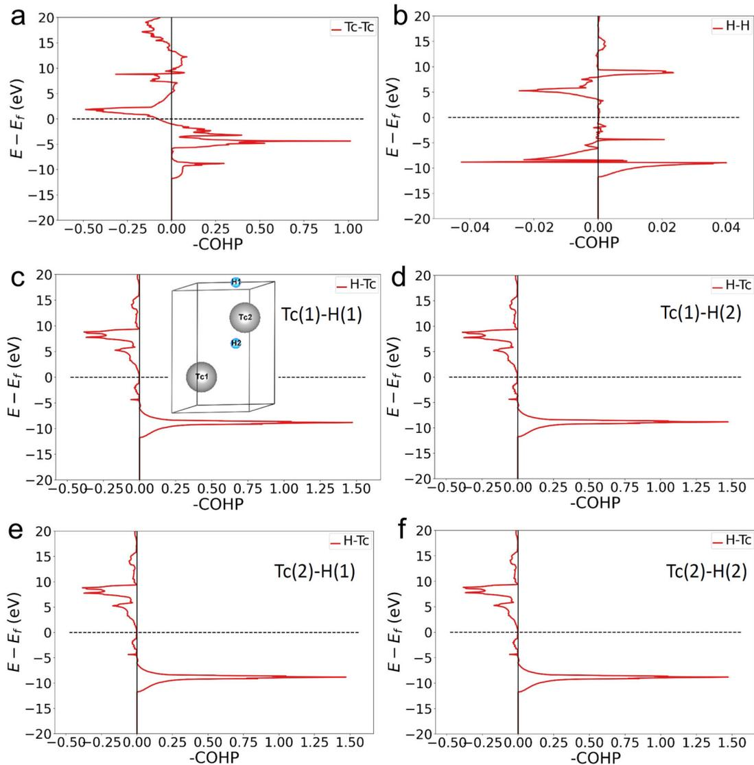
**Figure S10.** The Crystal Orbital Hamilton Population (COHP) analysis of bonding in *hcp*-TcH at 25 GPa. The calculations were performed using the Lobster code.<sup>28</sup>
