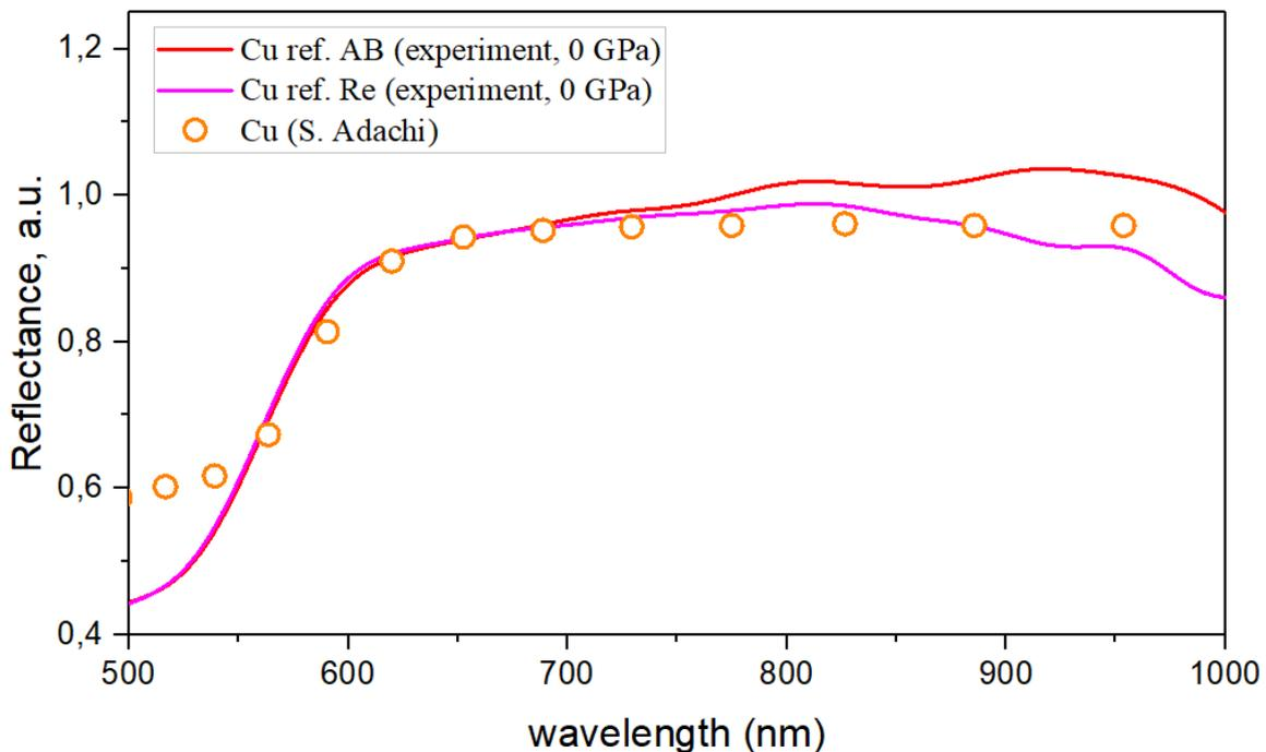
**Figure S26.** Reflectance of copper (Cu) obtained by dividing  $I_{\text{Cu}}(\lambda)$  by the reflection from the AB/diamond boundary (red) and from the rhenium gasket (Re, violet), which were used as reference points. The literature data for Cu<sup>30</sup> is shown by orange circles. A constant of 1/1.05 was used to correct the obtained value of  $I_{\text{Cu}}(\lambda)/I_{\text{ref}}(\lambda)$ . A sharp decrease in the Cu reflectivity below 600 nm is well reproduced in the experiment.
