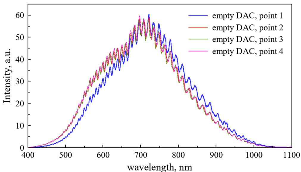
**Figure S18.** Transmission spectra of an empty diamond anvil cell measured at different points (1–4) of the diamond anvil culet. A strong interference component is present in the spectra.
