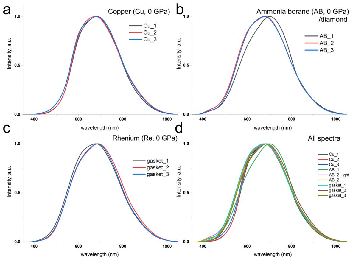
**Figure S24.** Fourier-filtered reflectance spectra, normalized to a unity, of (a) a copper particle loaded together with (b) ammonia borane (AB), and (c) rhenium gasket; (d) all spectra shown together. In panel (b),  $R(\lambda)$  at point 1 obviously deviates from the behavior of the material at other points, therefore point 1 was excluded from further analysis.
