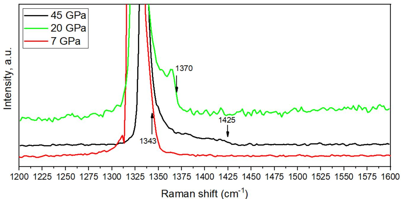
**Figure S12.** Raman spectra of the  $\text{TcH}_x$  samples taken at different pressures in the range of 1200–1600  $\text{cm}^{-1}$  (pressure determination).
