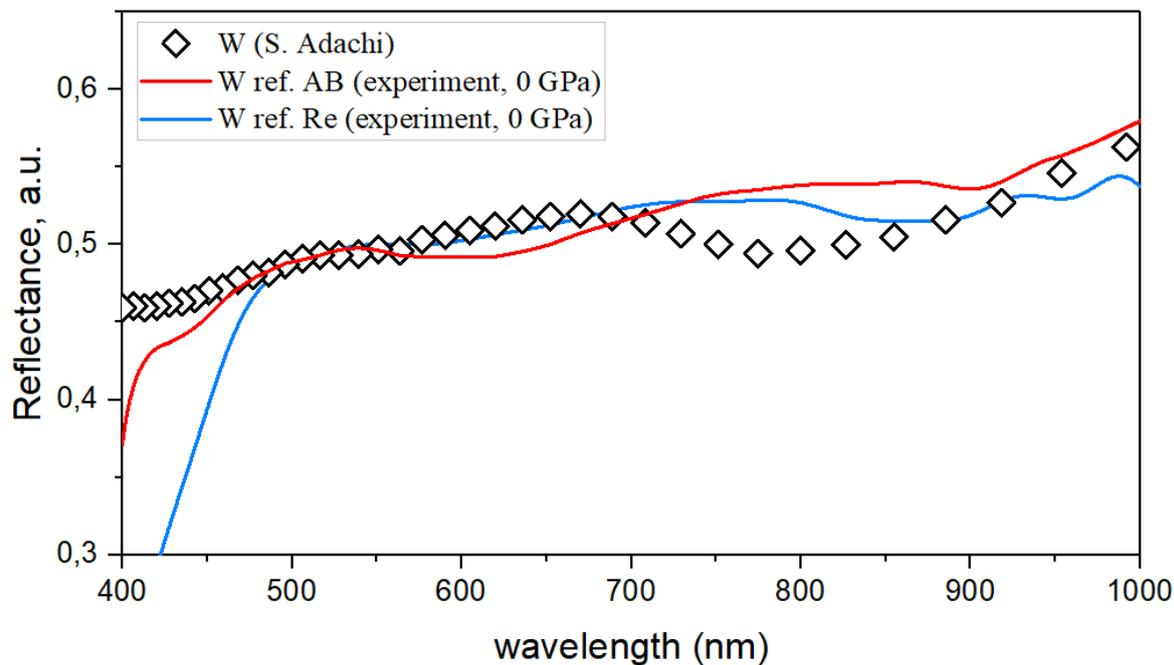
**Figure S27.** Reflectance of tungsten (W) obtained by dividing  $I_W(\lambda)$  by the reflection from the AB/diamond boundary (red) and from the rhenium gasket (Re, blue), which were used as reference points. The literature data for W<sup>30</sup> is shown by hollow diamonds. A general trend of decreasing reflectivity of W below 0.5 when moving from 1000 nm to 400 nm is reproduced in our experiment, but we could not detect a small local decrease around 750–800 nm.
