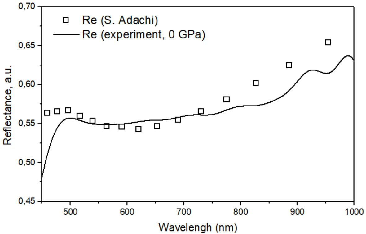
**Figure S25.** Reflectance of rhenium (Re) obtained by averaging the experiments on reflection from the gasket at 0 GPa, compared with the literature data.<sup>30</sup> The reflection from the diamond/ammonia borane (AB) boundary was used as the reference point. A constant of 1/1.8 was used to correct the obtained value of  $I_{\text{Re}}(\lambda)/I_{\text{AB}}(\lambda)$ . Upward trends at 500–600 nm and 700–1000 nm are qualitatively reproducible in the experiment.
