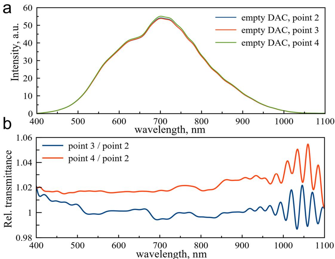
**Figure S20.** (a) Fourier-filtered transmittance spectra of the empty diamond anvil cell measured at different points (1–4, Figure S17) of the diamond anvil culet. All points except point 1 give almost identical transmittance spectra. This calibration experiment shows the importance of accumulating sufficient statistics on the transmittance spectra to draw certain conclusions. (b) Relative transmittance ( $I_{\text{sample}}/I_{\text{ref}}$ ) of the DAC in points 3,4 with respect to point 2.
