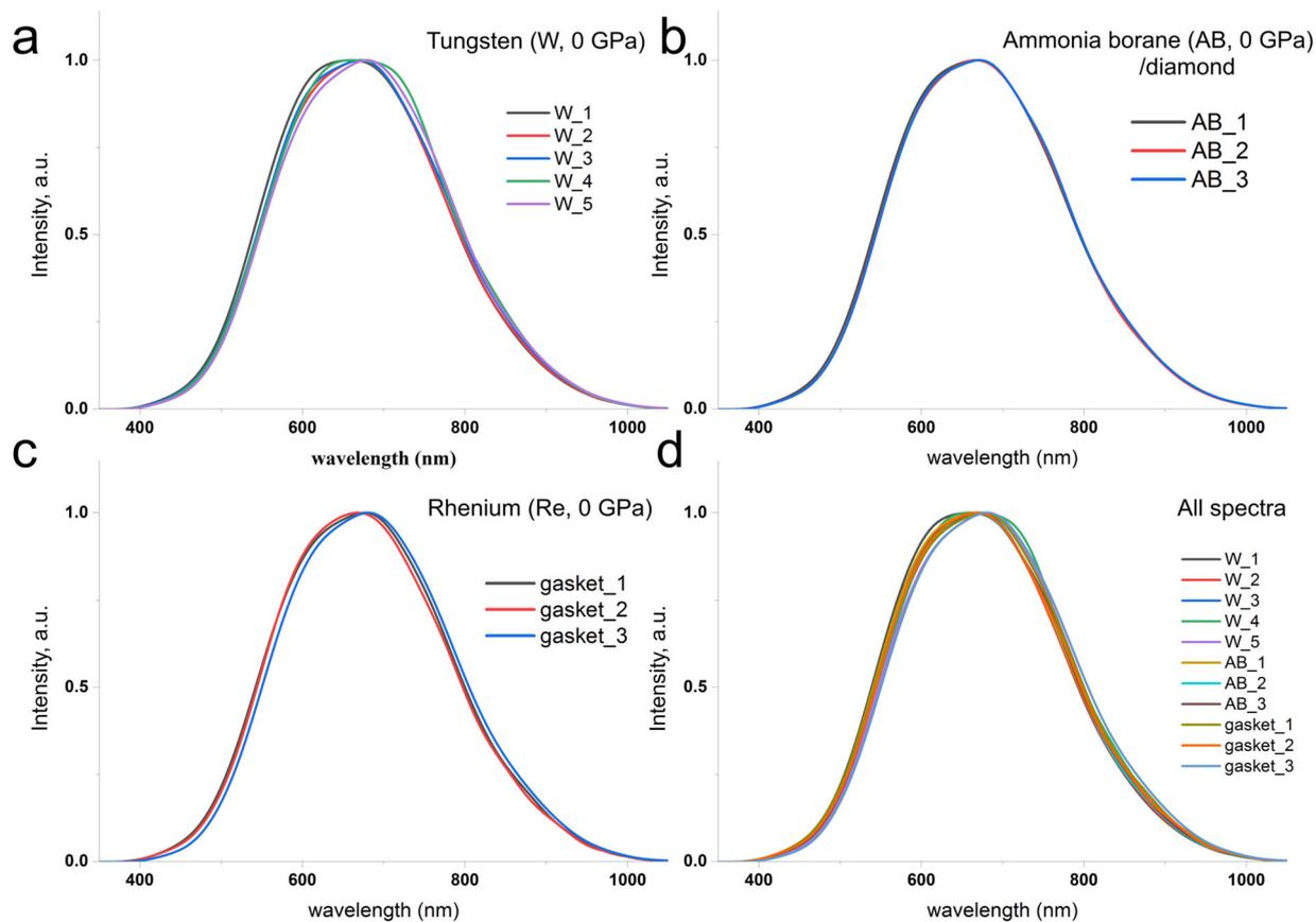
**Figure S23.** Fourier-filtered reflectance spectra, normalized to a unity, of (a) a tungsten particle loaded together with (b) ammonia borane (AB), and (c) rhenium gasket; (d) all spectra shown together.
