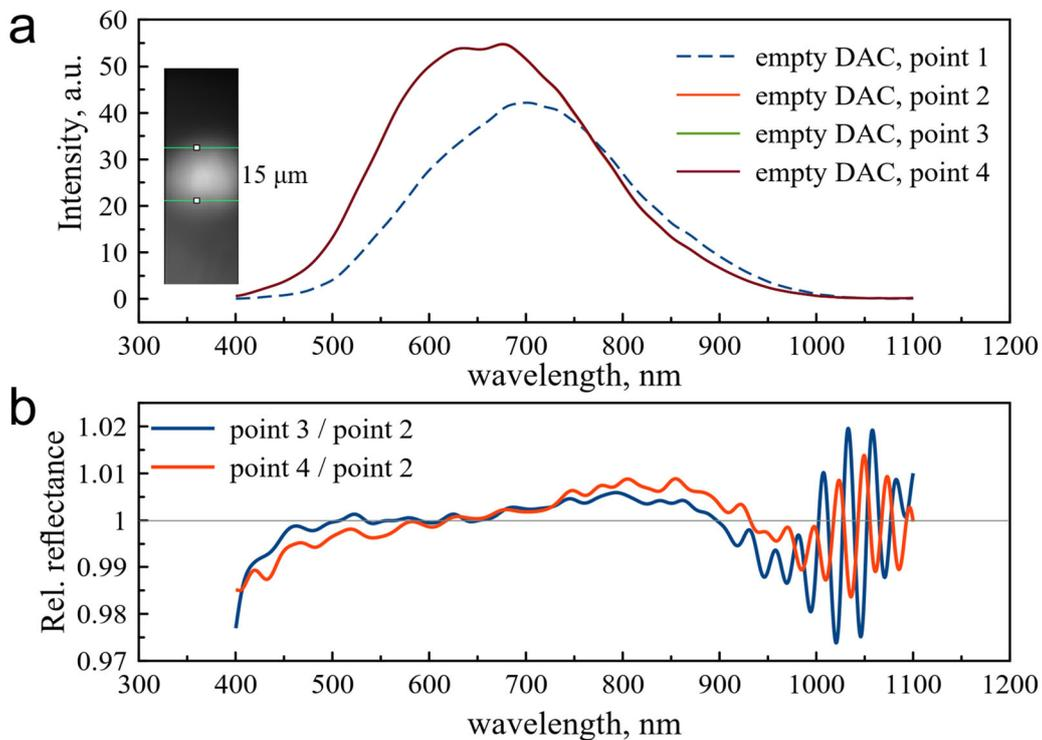
**Figure S19.** (a) Fourier-filtered reflectance spectra of the empty diamond anvil cell measured at different points (1–4, Figure S16) of the diamond anvil culet. All points except point 1 give almost identical reflectance spectra. This calibration experiment shows the importance of accumulating sufficient statistics on the reflectance spectra to draw certain conclusions. (b) Relative reflectance ( $I_{\text{sample}}/I_{\text{ref}}$ ) of the DAC in points 3,4 with respect to point 2.
