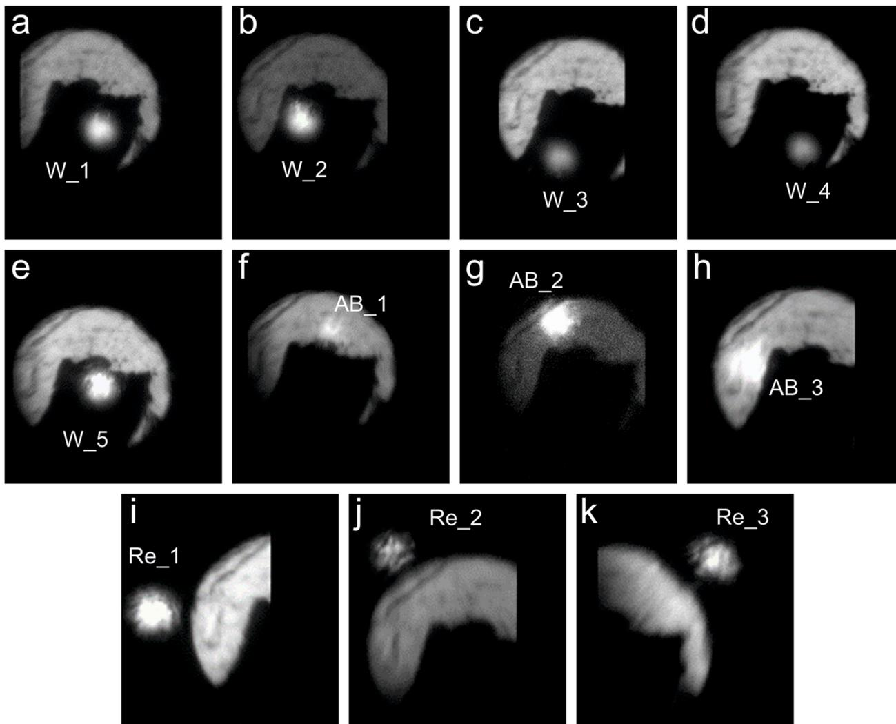
**Figure S15.** Optical photographs of a tungsten (W, a-e) sample placed in a high-pressure diamond anvil cell in a medium of ammonia borane (AB, f-h) equipped with a rhenium (Re, i-k) gasket. The bright spot of light (~15-20  $\mu\text{m}$ ) corresponds to the area where the measurements were made.
