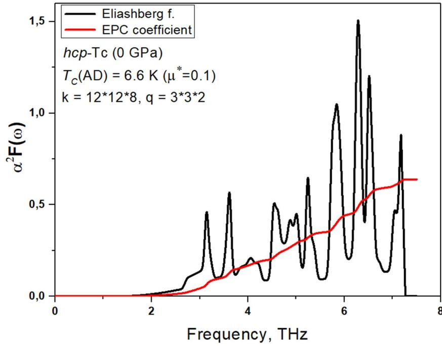
**Figure S9.** Eliashberg function and electron–phonon interaction parameter( $\lambda$ ) for *hcp*-Tc technetium at 0 GPa calculated using the Quantum Espresso code with the PBE functional and HGH-type pseudopotential.<sup>26,27</sup>
