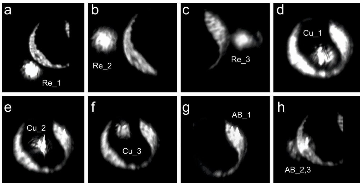
**Figure S14.** Optical photographs of the copper (Cu, d-f) sample placed in a high-pressure diamond anvil cell in a medium of ammonia borane (AB, g-h) equipped with a rhenium (Re, a-c) gasket. The bright spot of light ( $\sim$ 15-20  $\mu$ m) corresponds to the area where the measurements were made.
