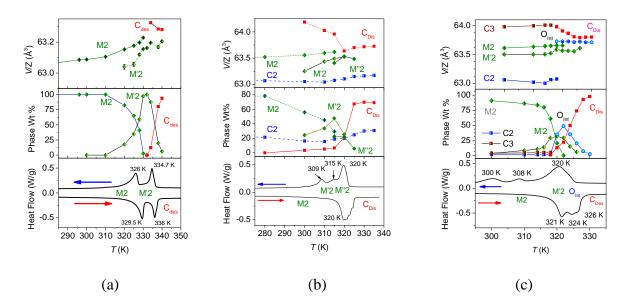
**Fig. 6.** Cell volume, weight percentage and DSC curve of (a)  $Y_{0.9}Gd_{0.1}Fe_2D_{4.2}$  (DEUT-M2) and  $Y_{0.9}Gd_{0.1}Fe_2H_{4.2}$  (b) (HYD-M2-A) and (c) (HYD-M2-B) compounds.
