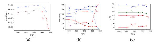
**Fig. 8.** a) Reduced cell volumes of C3, O and  $C_{Dis}$  phases, b) weight percentage of C3, O, and  $C_{Dis}$  phases upon heating and M1 and C2 upon cooling (c) cell parameters of C3 and O upon heating.
