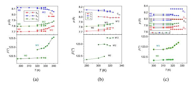
**Fig. 7**. Cell parameters (*p*) and monoclinic angle evolution of the M2, M'2, O and C2, C3 and C<sub>Dis</sub> phases in (a) DEUT-M2, (b) HYD-M2-A and (c) HYD-M2-B compounds.
