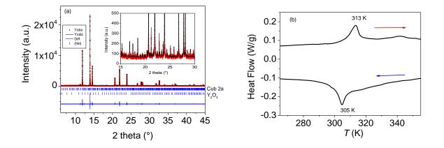
**Fig. 5.** (a) Pattern matching refinement of the  $Y_{0.9}Gd_{0.1}Fe_2H_{3.9}$  pattern measured at 140 K using *P*-43*m* SG, (b) DSC curve.
