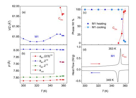
**Fig. 4.** (a) Cell volume (V/Z), (b) Cell parameters (p), (c) phase percentage and (d) DSC curve of  $Y_{0.9}Gd_{0.1}Fe_2H_{3.35}$  (HYD-M1).
