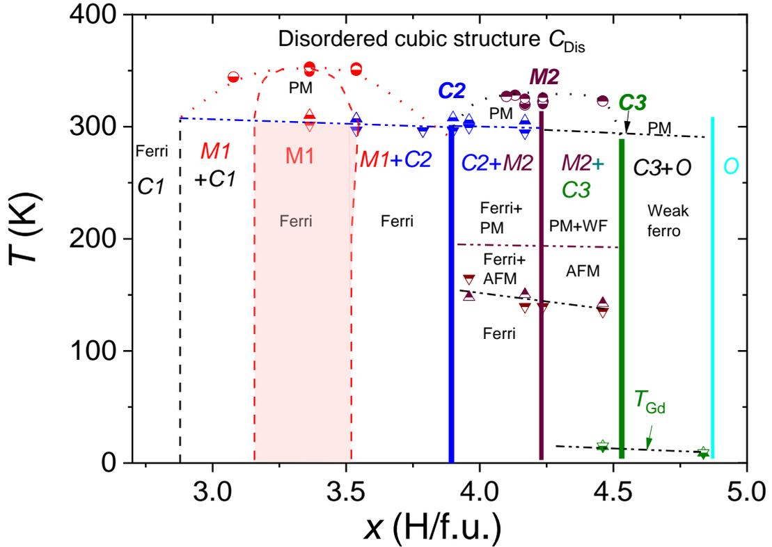
**Fig. 6:** Schematic structural and magnetic phase diagram of  $Y_{0.9}Gd_{0.1}Fe_2H_x$  hydrides with *C1* (black), *M1* (red), *C2* (blue), *M2* (brown), *C3* (olive) and *O* (cyan) phases. The magnetic transitions are indicated with triangles (up: heating and down: cooling) whereas the O-D transitions are indicated by circles ( $\blacklozenge$ : heating and  $\blacklozenge$ : cooling).
