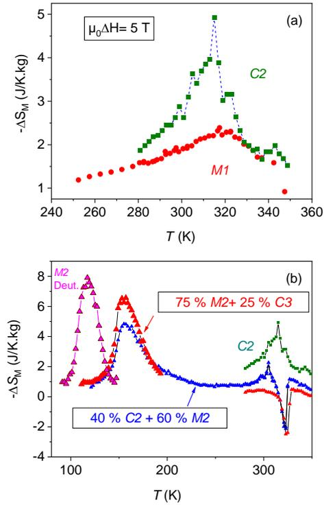
**Fig. 7:** Magnetic entropy variation  $\Delta S_M$  versus temperature for different hydrides with a field variation  $\mu_0\Delta H = 5$  T. (a) for *M1* and *C2* single phases and (b) for samples containing *M2* including a monoclinic  $Y_{0.9}Gd_{0.1}Fe_2D_{4.2}$  deuteride which is added for comparison.
