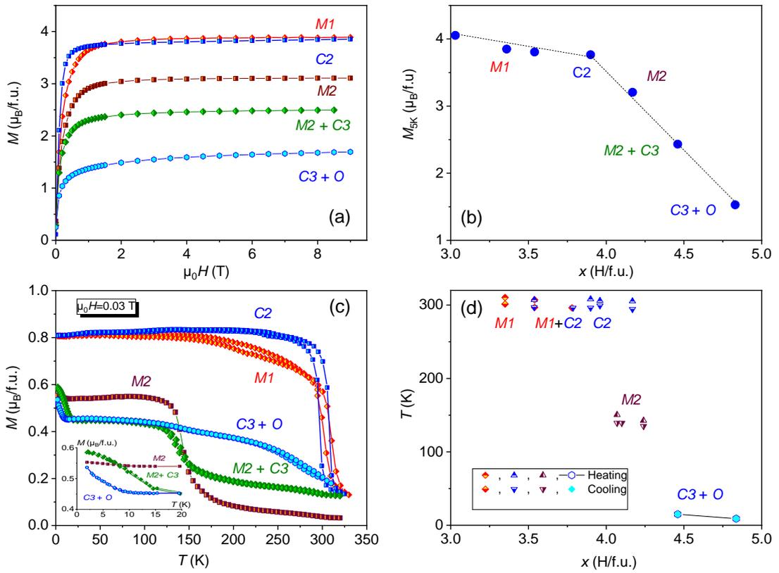
**Fig. 2:** (a)  $M_{5K}(B)$  and (b) magnetization at 5 K, (c)  $M_{0.03T}(T)$  and (d) magnetic transition temperatures versus *H* concentration of  $Y_{0.9}Gd_{0.1}Fe_2H_x$  hydrides. Two samples presented in (a) and (c) contain a mixture of two phases: 31 % *M2*+ 69% *C3* (*M2*+*C3*) and 20% *C3*+80% *O* (*C3*+*O*). Inset (c): zoom below 20 K.
