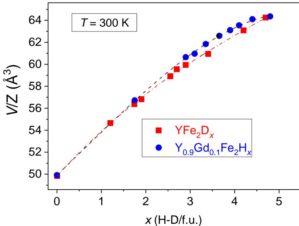
**Fig. 1.** Cell volume swelling of  $Y_{0.9}Gd_{0.1}Fe_2H_x$  and  $YFe_2D_x$  compounds at 300 K. The error bars are smaller than the symbols. The curves have been fitted by a polynomial function.
