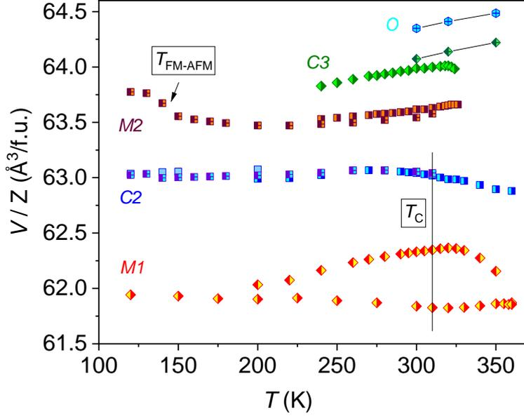
**Fig. 5:** Cell volume evolution versus temperature of the different phases below the O-D transitions measured for several samples. The magnetic transitions temperatures ( $T_{FM-AFM}$  and  $T_C$ ) are indicated in box. The two different  $V/Z$  variations of  $M1$ , reflect the large solubility range: the lower one corresponds to a single  $M1$  phase whereas the upper one was measured for a mixture of  $M1 + C2$ .
