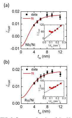
FIG. 3.  $\xi_{FMR}$  as a function of the thickness of Ni ( $t_{Ni}$ ) in Nb/Ni (a) and Ru/Ni (b) bilayers. The inset shows a plot of  $1/\xi_{FMR}$ against  $1/t_{Ni}$ . The red continuous line is the fit using equation (1).
