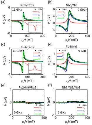
Fig. 2. Experimentally measured ST-FMR data in Nb(5 nm)/Fe<sub>60</sub>Co<sub>20</sub>B<sub>20</sub>(FCB) (5 nm) (a), Nb (5 nm)/Ni (6 nm) (b), Ru (4 nm)/FCB (5 nm) (c), Ru (4 nm)/Ni (6 nm) (d), Ru (2 nm)/Ni (6 nm)/Ru (2 nm) (e) and Nb (3 nm)/Ni (6 nm)/Nb (3 nm) (f). Black points are the experimental data which is fit to the green curve that is the sum of  $V_S$  (red curve),  $V_A$  (blue curve) and a constant dc offset.
