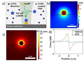
Fig. 1. a) Schematic of plasmon-assisted Opto-thermoelectric trapping of fluorescent nanodiamonds on Gold Nanoparticles. The surfactant (CTAC) facilitates an electric field which attracts the FND to AuNP. b) & c) Simulated temperature and temperature gradient distributions for a 400 nm AuNP placed on a glass substrate and surrounded by water. d) Comparison of opto-thermoelectric (OTE) and optical force in our geometry showing OTE force dominates the trapping.
