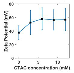
Fig. S3. Zeta potential of FNDs plotted as a function of concentration of CTAC.
