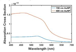
Fig. S1. Calculated absorption cross section of the drop-casted Au np (150 and 400 nm diameter).
