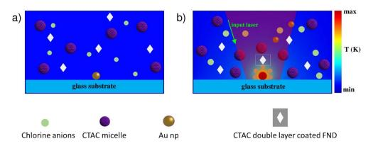
Fig. S2. Mechanism of reversible trapping of FND using single nanoparticle driven optothermoelectric trap. a) Gold particles are drop-casted and aqueous solution of fluorescent nanodiamonds with surfactant is added. b) Laser on Au np creates a thermal gradient driving the trapping.
