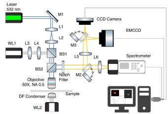
Fig. 2. Optical schematic of the trapping setup including lenses (L), mirrors (M), beam splitters (BS), white light sources (WL), 50x objective lens of 0.5 numerical aperture, a dark field (DF) condenser of numerical aperture 1.4, a charge-coupled device (CCD) camera, an electron multiplying CCD (EMCCD) camera, and a spectrometer. This scheme integrates dark-field microscopy, optical spectroscopy, tracking, and fluorescent imaging.
