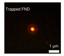
Fig. S8. Fluorescence image of single optically trapped FND using a water immersion objective lens (NA 1.2).
