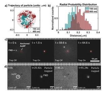
Fig. 3. a) Trajectories of trapped FND using 150 nm and 400 nm diameter AuNPs. The corresponding radial probability distribution shown in c) shows that the trapped FNDs radial distribution varies with the diameter of the anchor particle. Snapshots of single FND trapping are shown for c) 150 nm AuNP (See Visualization 1 and 2), d) 400 nm AuNP (See Visualization 3). The times series fluorescent images show the trap and release ability of a single FND.
