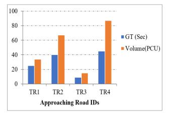
Fig. 10(b) Allocated green time v/s PCU at THC
