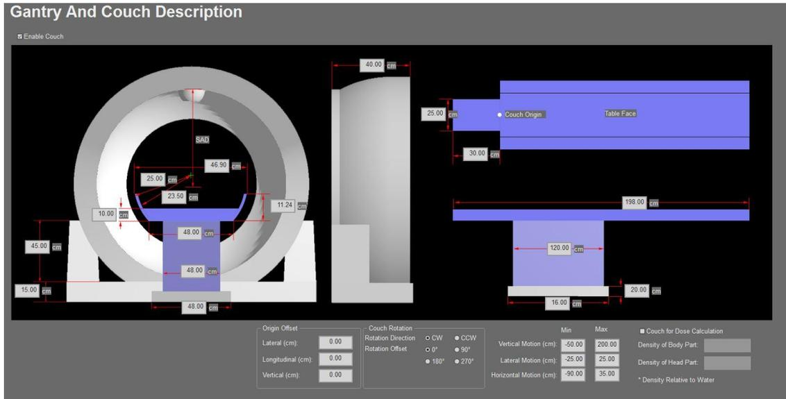
**Figure 3.** Detailed blueprint for the gantry and couch in the Galaxy system.
