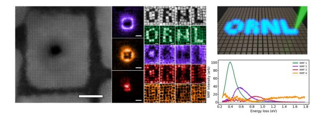
**Figure 4.** Electron beam sculpting of matter and its connection to its nanophotonic properties. Specific energetic features can be placed by the electron beam by sculpting nanoparticles into geometric shapes that support a desired nanophotonic property. Reprinted with permission from John Wiley and Sons.
