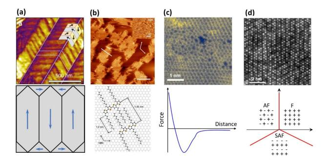
**Figure 7.** (a) Force-SPM phase image shows domain structure in PbZr0.2Ti0.8O3.Adapted with permission from ref<sup>220</sup> (b) Force-SPM images of P3DT adsorbed on the surface of hBN. Adapted with permission from ref<sup>221</sup> (c) STEM image of disordered graphene, , and force-distance curve. (d) STEM of a MoS<sub>2</sub>doped with Re atoms, adapted with permission from Ref<sup>222</sup> with a snapshot of the Ising model.
