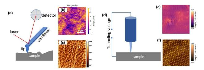
**Figure 3.** Overview of the scanning probe microscopy (SPM) operation, which includes force-SPM and scanning tunnelling microscopy (STM), (a) schematic of the force-SPM setup, (b), force-SPM topography image, adapted with permission from ref<sup>60</sup>, (c), force-SPM resonance frequency image, adapted with permission from ref<sup>70</sup>. (d) schematic of STM setup, (e, f), STM images of atomic defects in graphene (e) and molecular self-assembly (f).
