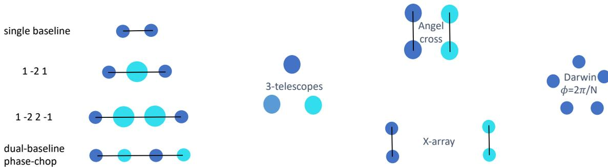
Figure 4. A (partial) catalog of nulling interferometry configurations from the literature.
