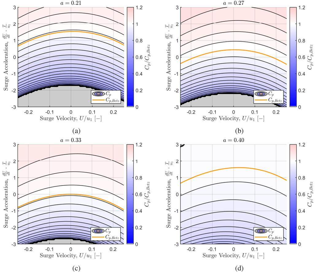
Figure 16: Contours of  $C_p / C_{p,Betz}$  for a moving porous asymmetric body (parameterized by Equation 5.20), plotted in the surge-kinematics phase plane as a function of surge velocity and acceleration for induction factors of (a) 0.21, (b) 0.27, (c) 1/3, and (d) 0.40. The orange line indicates  $C_p = C_{p,Betz}$ , and grey regions denote dynamics that violate one or more assumptions of the theoretical framework.
