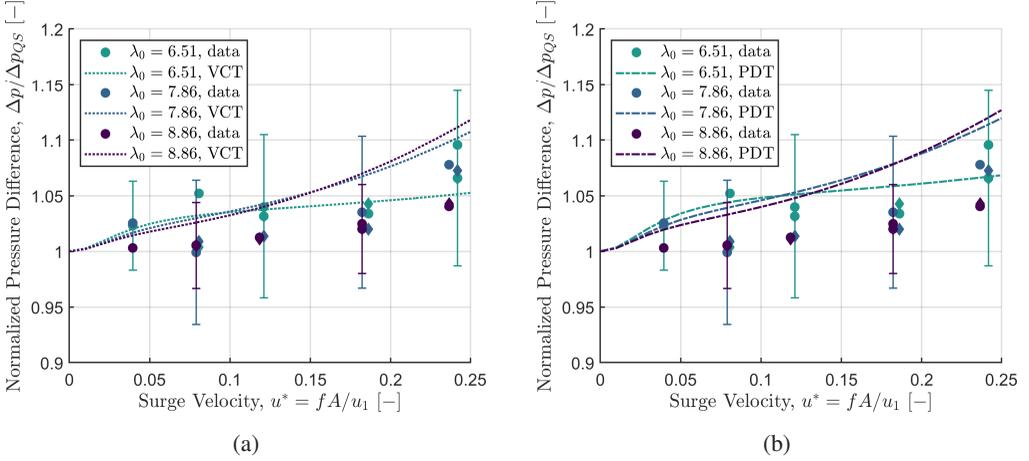
Figure 13: Pressure difference across the turbine,  $\Delta p = p(x = x_u) - p(x = x_d)$ , normalized by the quasi-steady pressure difference and plotted against surge-velocity amplitude. Model predictions are given as dotted lines for the VCT model in (a) and as dashed-dotted lines for the PDT model in (b). Error bars are shown on every fourth point.
