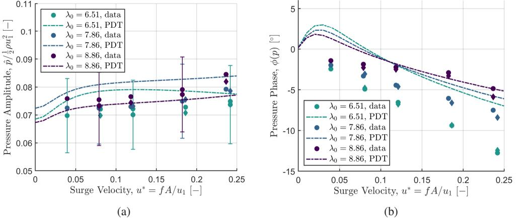
Figure 12: (a) Amplitude and (b) phase of the measured relative pressure at  $x = x_u$ , plotted against surge-velocity amplitude. PDT model predictions are given as dashed-dotted lines. Error bars are plotted on every fourth point.
