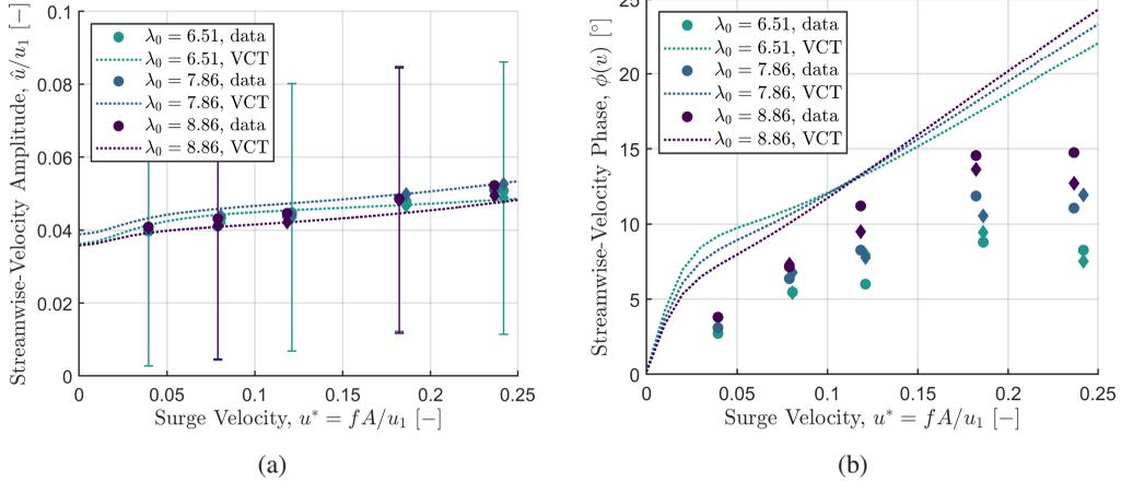
Figure 18: (a) Amplitude and (b) phase of the measured flow velocity at  $x = x_u$ , plotted against surge-velocity amplitude. VCT model predictions are given as dotted lines. Error bars are plotted on every fourth point.
