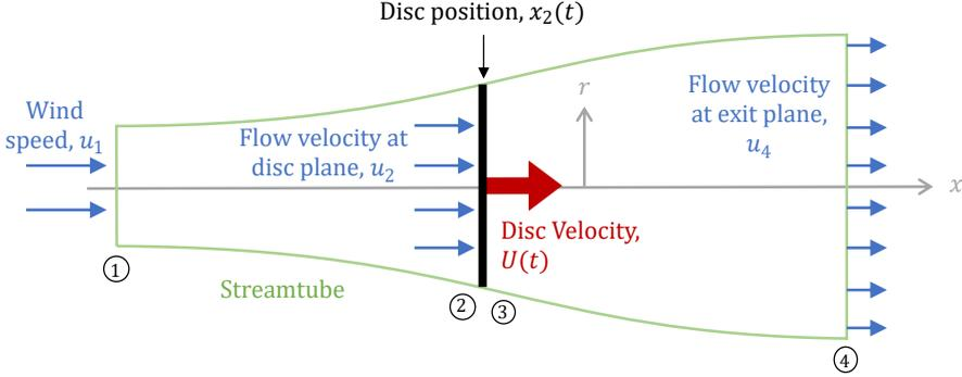
Figure 1: Schematic of the parameters and control volumes referenced in Section 2. The actuator disc is located instantaneously at  $x_2(t)$  and moves with velocity  $U(t)$  relative to the inertial frame defined by the  $x$ - and  $r$ -axes. Circled numbers denote streamwise interrogation locations (1 through 4).
