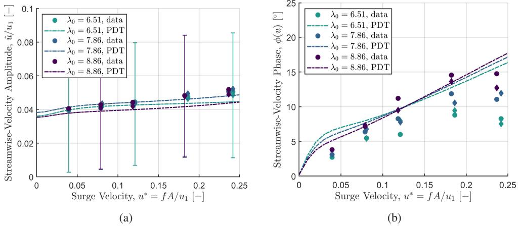
Figure 11: (a) Amplitude and (b) phase of the measured flow velocity at  $x = x_u$ , plotted against surge-velocity amplitude. PDT model predictions are given as dashed-dotted lines. Error bars are plotted on every fourth point for clarity.
