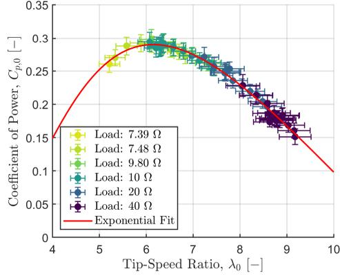
Figure 3: Steady power curve for the turbine used in these experiments, measured over a range of resistive loads and wind speeds. Some of these data points are reproduced from [Wei & Dabiri \(2022\)](#). The result of the exponential fit given by Equation 3.1 is shown as a solid red line.
