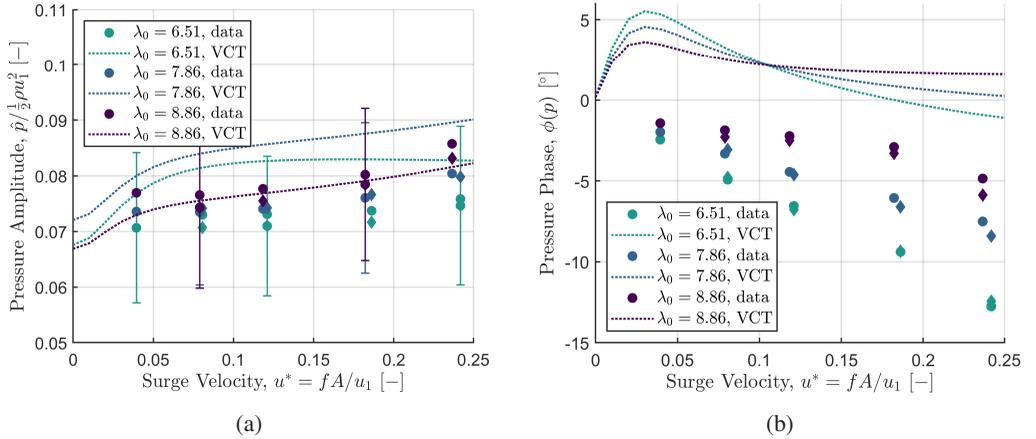
Figure 19: (a) Amplitude and (b) phase of the measured relative pressure at  $x = x_u$ , plotted against surge-velocity amplitude. VCT model predictions are given as dotted lines. Error bars are plotted on every fourth point.
