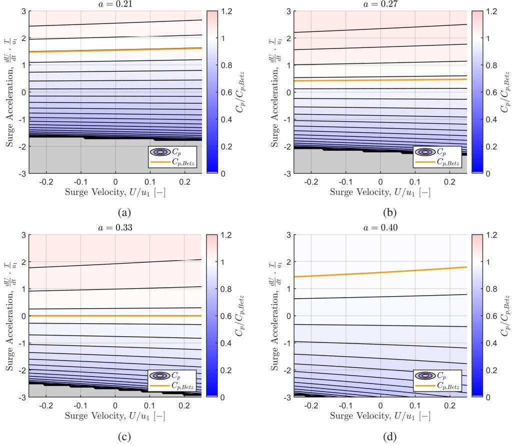
Figure 15: Contours of  $C_p/C_{p,Betz}$  calculated from Equation 5.14 for a moving porous disc, plotted in the surge-kinematics phase plane as a function of surge velocity and acceleration for induction factors of (a) 0.21, (b) 0.27, (c) 1/3, and (d) 0.40. The orange line indicates  $C_p = C_{p,Betz}$ , and grey regions denote dynamics that violate one or more assumptions of the theoretical framework. To nondimensionalize the surge acceleration,  $T$  is taken to be 1 s.
