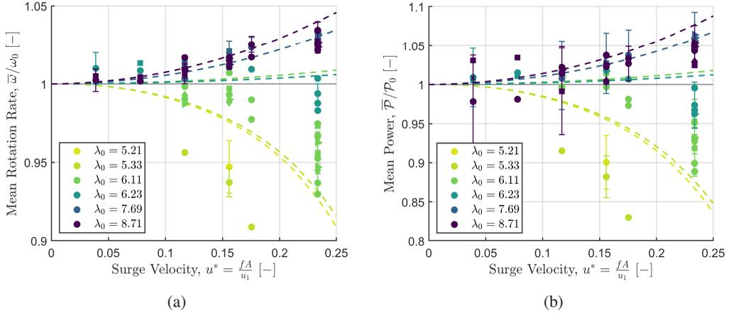
Figure 7: Time-averaged (a) rotation rate and (b) power, plotted against surge-velocity amplitude. Data are reproduced from [Wei & Dabiri \(2022\)](#); model predictions derived from Equation 2.7 are plotted as dashed lines and colored by tip-speed ratio. Circles represent sinusoidal surge-velocity waveforms and diamonds and other markers represent trapezoidal waveforms. Error bars are plotted on every sixth point for the sake of clarity.
