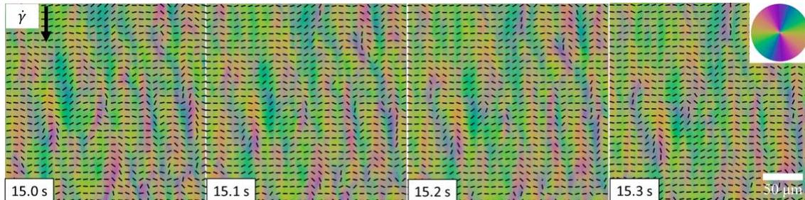
Fig. 7. Time evolution of the director field of a sheared DSCG mapped by a PPM. The arrow points along the shearing direction.  $\dot{\gamma} = 22.5 \text{ s}^{-1}$ ,  $d = 10 \text{ }\mu\text{m}$ ,  $T = 24^\circ\text{C}$ .
