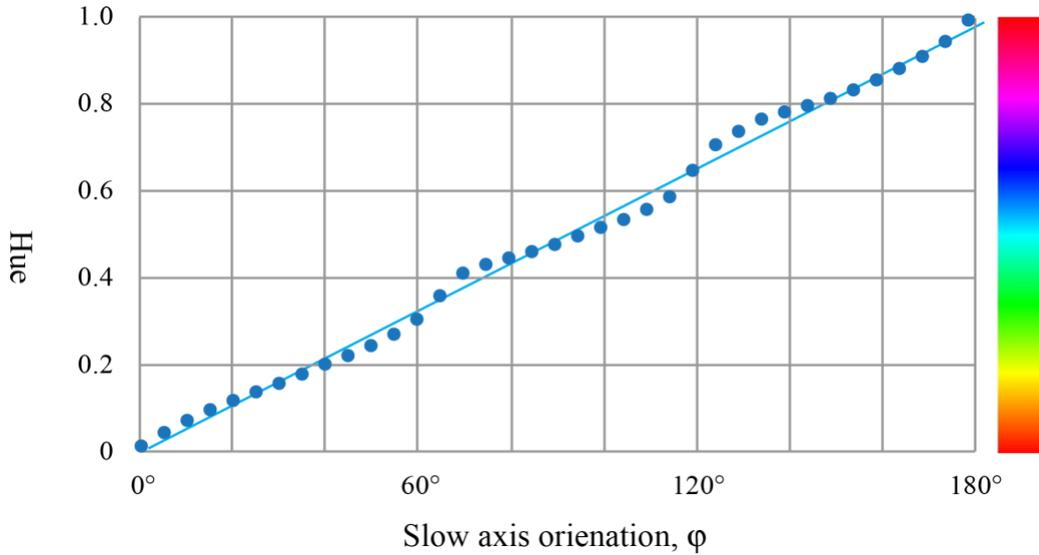
Fig. 3. Dependence of the hue on the slow axis orientation of a 154-nm retardance waveplate. The hue bar is shown on the right in color.
