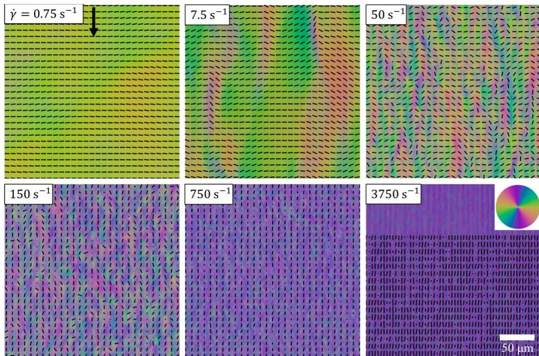
Fig. 6. PPM maps the director orientation of DSCG under different shearing rates. The arrow points along the shearing direction.  $d = 10 \mu\text{m}$ ,  $T = 24^{\circ}\text{C}$ . In the panel for  $3750 \text{ s}^{-1}$  the top stripe is intentionally left without the director pattern to demonstrate the periodic nature of distortions.
