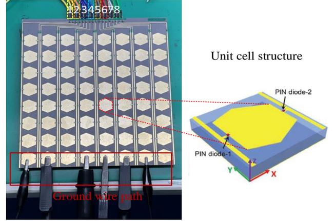
Fig. 10: Photograph of the 4<sup>#</sup> 2-bit RIS.
