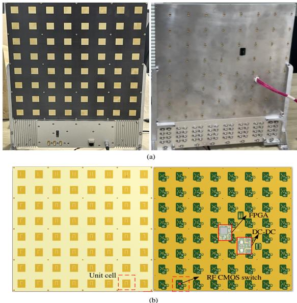
Fig. 15: Photograph of the 6<sup>#</sup> fabricated RF switch-based RIS. (a) The front and back structure of RIS. (b). The physical structure of RIS.
