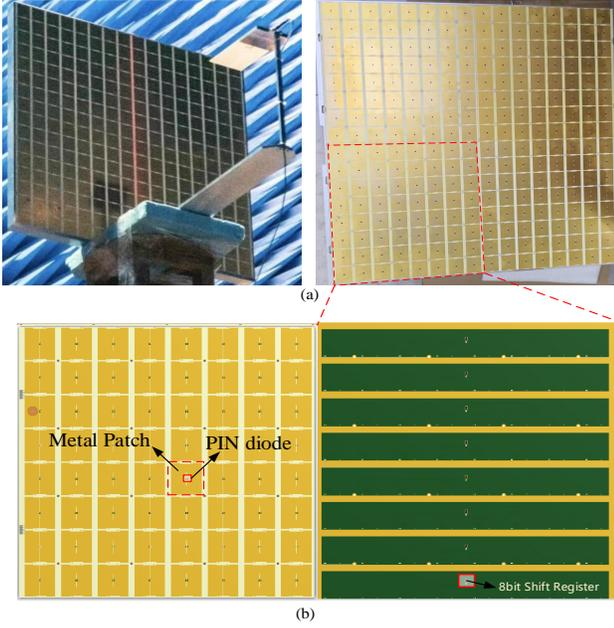
Fig. 3: Photograph of the fabricated 1<sup>#</sup> PIN-diode-based RIS. (a) A complete  $16 \times 16$  RIS. (b) An  $8 \times 8$  sub-RIS structure.
