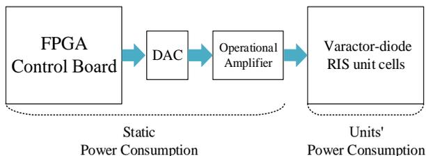
Fig. 14: The fabricated varactor-diode-based RIS hardware design structure.
