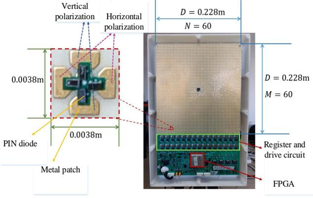
Fig. 5: Photograph of the 2<sup>#</sup> dual-polarized PIN-diode based RIS.
