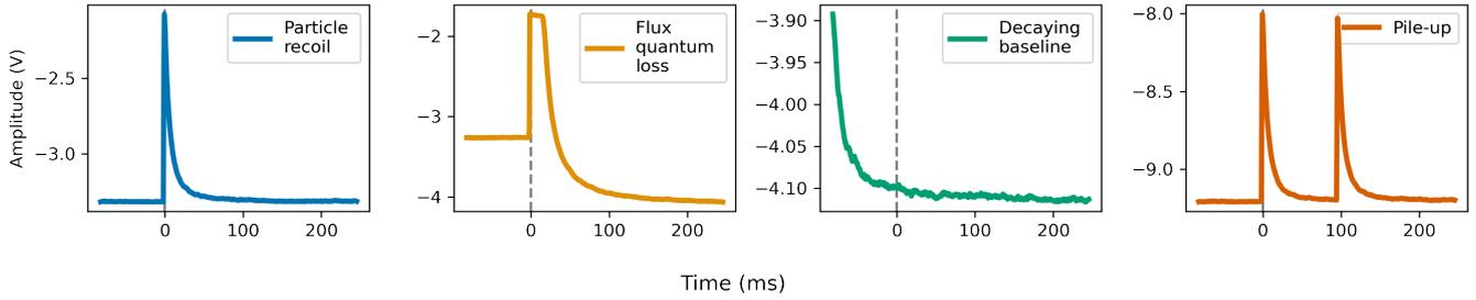
**Fig. 1.** Particle recoils produce a pulse-shaped record (blue). Flux quantum losses of the SQUID amplifier in the read-out circuit are caused by fast magnetic field changes, e.g. from high energy recoils (orange). Decaying BLs are residuals from earlier high energy pulses (green). Pile-up originates from multiple particle recoils within the same record window (red).
