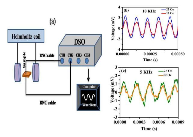
**Fig.5**. (a) Schematic diagram of BFO\_P(VDF-TrFE) ME sensor; (b) and (c) Voltage response of 1.5 vol % BFO\_P(VDF-TrFE) nanocomposite film at 25 and 12 Oe AC magnetic field for 10 kHz and 5 kHz, respectively.
