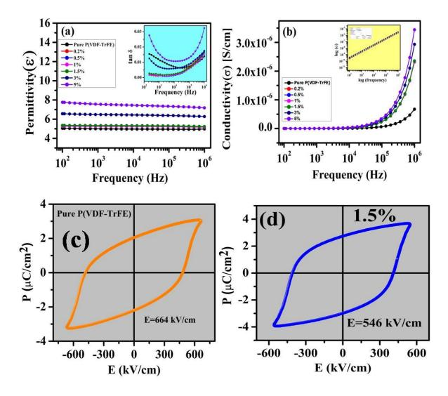
**Fig.2.** Frequency dependent (a) dielectric permittivity and (inset: loss tangent versus frequency) and (b) conductivity versus frequency for pure P(VDF-TrFE) film and BiFeO<sub>3</sub>\_P(VDF-TrFE) nanocomposite films; Ferroelectric polarisation versus electric field curve for (c) pure P(VDF-TrFE) film and (d) 1.5 vol % BiFeO<sub>3</sub>\_P(VDF-TrFE)
