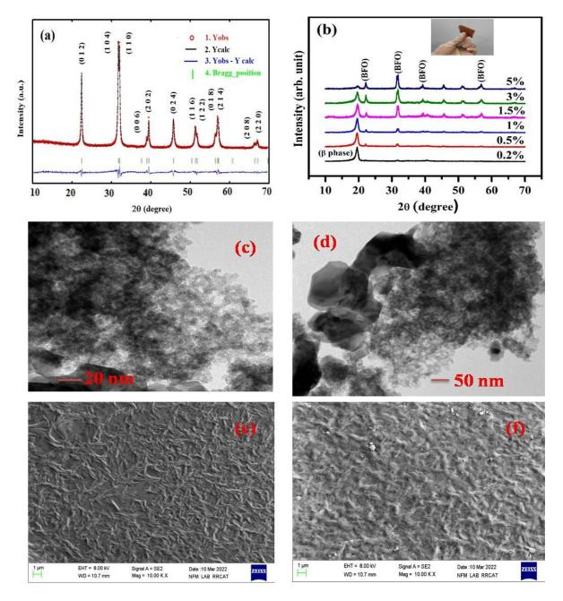
**Fig.1** (*a*) Rietveld refinement of BiFeO<sub>3</sub> nanoparticles; (*b*) XRD pattern of BiFeO<sub>3</sub>  $_{P}(VDF-TrFE)$  nanocomposite films (inset: photographic image of 1.5 vol % nanocomposite film); (*c*) and (*d*) TEM images of BiFeO<sub>3</sub> nanoparticles; FESEM images of (*e*) pure P(VDF-TrFE) and (*f*) 1.5 vol % BiFeO<sub>3</sub>  $_{P}(VDF-TrFE)$  nanocomposite film
