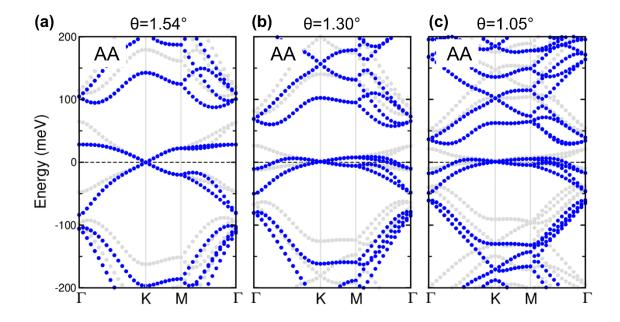
**Figure 3** Electronic band structures of twisted bilayer graphene with an intercalated charged defect ( $\tilde{q} = -0.1$ ) at the AA region for three twist angles: (a) 1.54°, (b) 1.30°, and (c) 1.05°. The band structure without the defect is shown in light grey for comparison. The zero of energy (indicated by the horizontal black dashed lines) is defined as the Dirac point energy.
