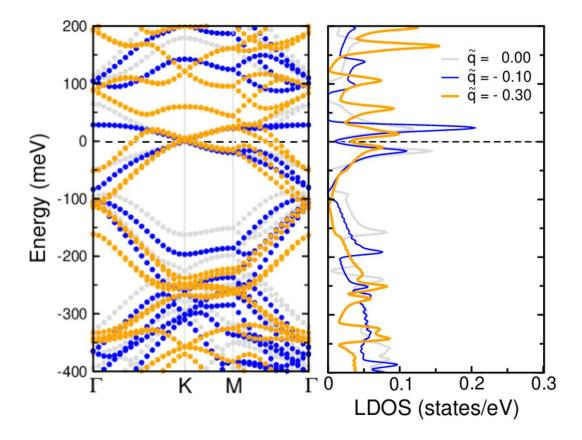
Figure 6 The local densities of states (LDOS) for tBLG with 1.54° twist angle for effective charges of 0.0, -0.10 and -0.30, intercalated at the AA region. The LDOS is calculated at a distance 2.93 nm away from the defect using 31 × 31 × 1 regular k-grid. The zero of energy is referenced to the energy of the Dirac point.
