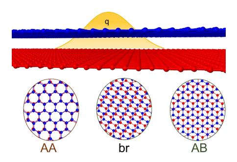
**Figure 1** Top: Schematic depiction of tBLG with the potential due to a charged defect (with charge q). Bottom: different high-symmetry stacking regions (AA, br, AB) that exist in the moiré unit cell of tBLG.
