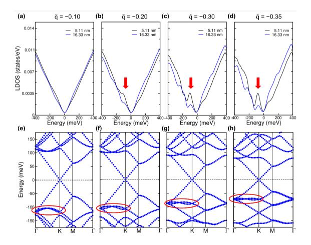
**Figure 4** (a)–(d) Local density of states of an 80 × 80 monolayer graphene supercell with a charged adsorbate for two distances from the defect and for four different values of the effective defect charge. Red arrows indicate the peak due to the collapse state. (e)–(h) Corresponding electronic band structures with the bands that give rise to the collapse state circled in red. The zero of energy is referenced to the energy of the Dirac point.
