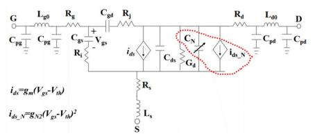
Fig.2 An approximation of the InP HEMT internal circuit by considering the nonlinearity effects illustration with a scribble-dotted line on the primary circuit.
