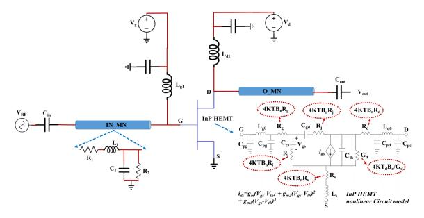
Fig. 1 the schematic of the circuit containing the input and output matching networks, stability network, and active elements (InP HEMT) and its internal circuit.
