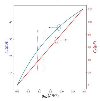
Fig. 5 InP HEMT DC characterization:  $I_{ds}$  (mA) vs.  $g_{N2}$  (A/V<sup>2</sup>), Nonlinear capacitance  $C_N$  (pF) vs.  $g_{N2}$  (A/V<sup>2</sup>)
