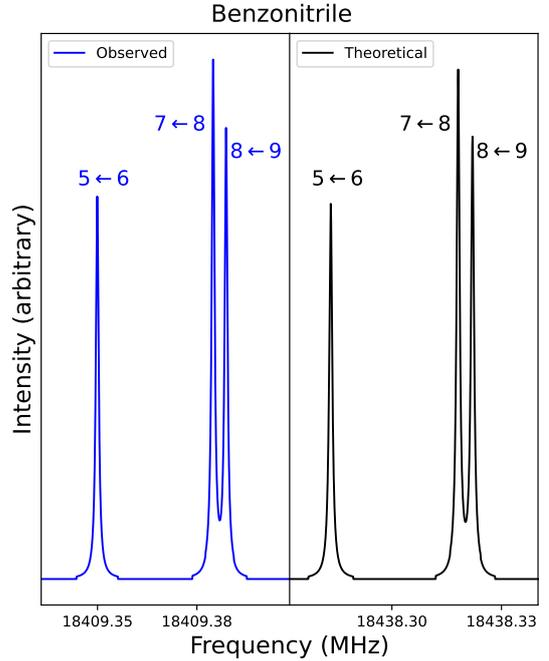
**Figure 3.**  $^{14}N$ -nuclear quadrupole hyperfine components of the  $7_{0,7} \rightarrow 6_{0,6}$  transition with  $F'' \rightarrow F'$  shown in blue and black colors for the observed and simulated benzonitrile transition, respectively, with the B3LYP/6-311+G(d,p) level.
