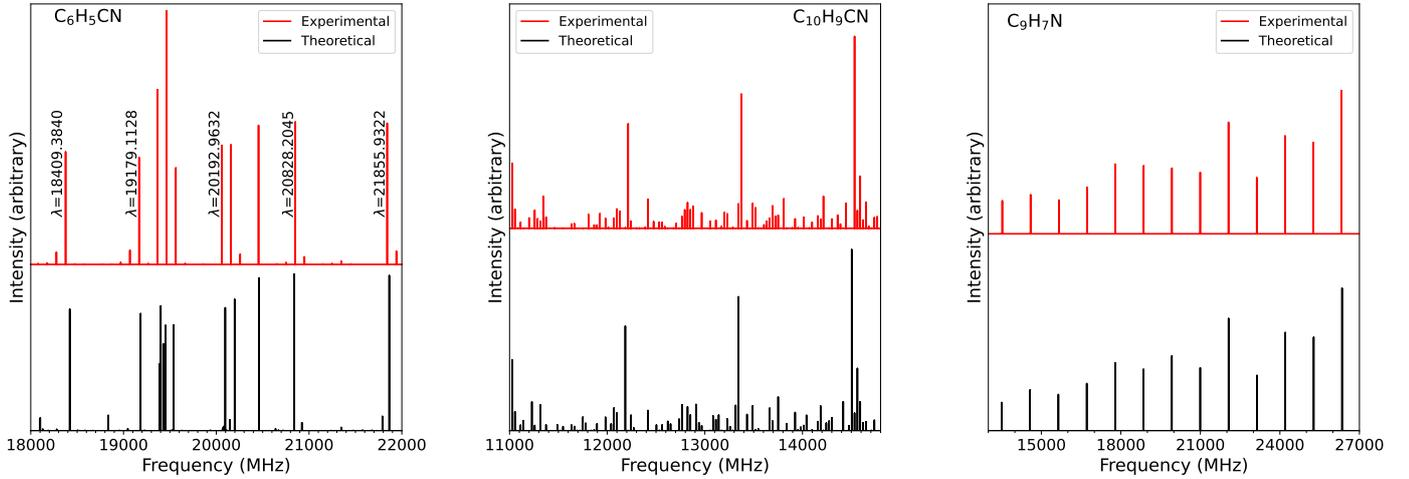
**Figure 2.** Rotational spectra of benzonitrile ( $C_6H_5CN$ ), 1-cyanonaphthalene ( $C_{10}H_7CN$ ) and quinoline ( $C_9H_7N$ ) with B3LYP/6-311+G(d,p) at 300 K (black) in the centimetre-wave region. The experimental spectra are shown in red. The band positions of detected emission lines of benzonitrile in the TMC-1 are labelled.
