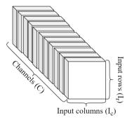
Figure 3 CNN input tensor.
