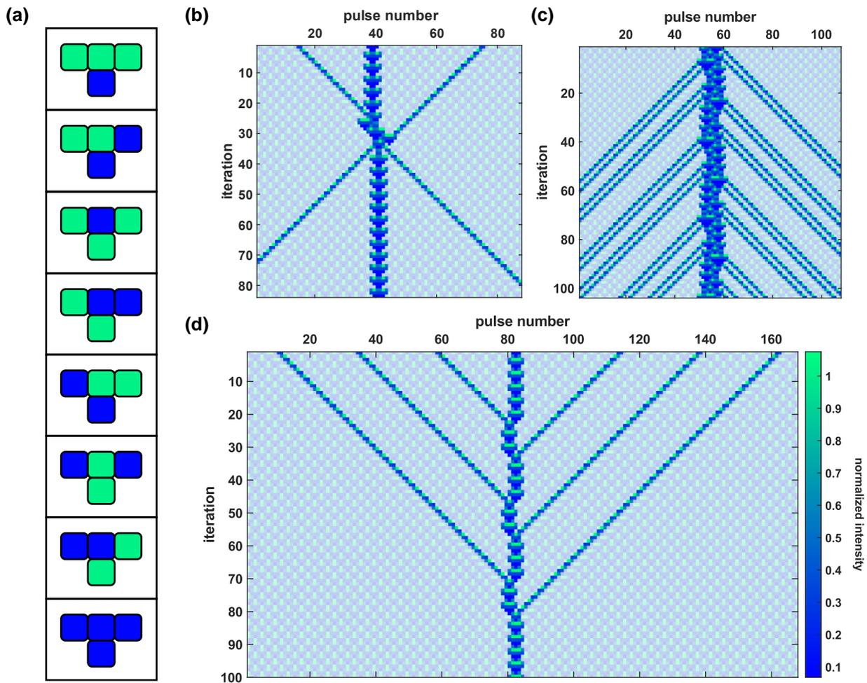
FIG. 4. **Soliton-like and glider interactions produced by ECA Rule 54 in the photonic hardware.** (a) Truth table showing the update for ECA Rule 54. Space-time diagrams of ECA Rule 54 with periodic background filtered out, showing (b) glider collision, (c) glider gun, and (d) black hole.
