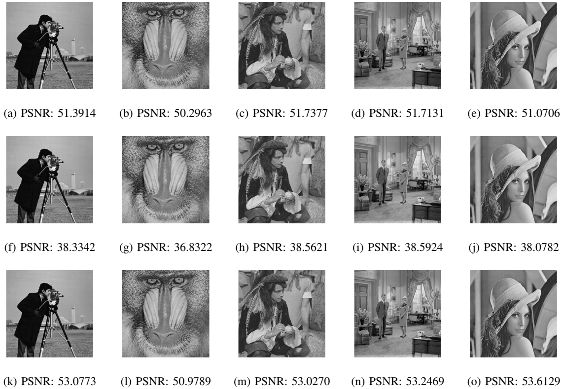
Fig. 13: Images obtained after DCT and IDCT using different CORDIC architectures (a)-(e): conventional CORDIC, (f)-(j): lookahead CORDIC and (k)-(o): RICO
