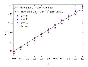
FIG. 7. Dependencies of the normalized electrical conductance on the proportions of rings and sticks, x, for the three different values of the number density of fillers,  $n_{\rm s}=xn$  and  $n_{\rm r}=(1-x)n$ , when  $n=2,\ n=5$ , and n=10. The MFA predictions (34) are shown as a line, while markers correspond to the simulations. Here,  $l=2\pi r,\ r=1,\ R_{\rm j}=1$ , and  $\rho_{\rm w}=(2\pi r)^{-1}10^{-6}$ .
