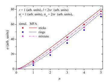
FIG. 3. Dependencies of the electrical conductance on the number density of fillers,  $n=n_{\rm s}+n_{\rm r}$ , when  $n_{\rm r}=0$ ,  $n_{\rm s}=n_{\rm r}$ , and  $n_{\rm s}=0$ . The MFA predictions are shown as curves, while markers correspond to the simulations. Here,  $l=2\pi r$ , r=1,  $R_{\rm j}=1$ , and  $\rho_{\rm w}=(2\pi r)^{-1}$ .
