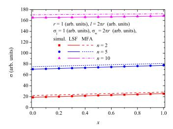
FIG. 4. Dependencies of the electrical conductance on the proportions of rings and sticks, x, for the three different values of the number density of fillers,  $n_{\rm s}=xn$  and  $n_{\rm r}=(1-x)n$ , when  $n=2,\ n=5$ , and n=10. MFA predictions and the least-squares fitting are shown as lines, while markers correspond to the simulations. Here,  $l=2\pi r,\ r=1,\ R_{\rm j}=1$ , and  $\rho_{\rm w}=(2\pi r)^{-1}$ .
