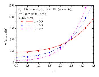
FIG. 9. Dependencies of the electrical conductance on the relative stick length, z, for the fixed values of the number density of fillers and different values of x. The MFA predictions are shown as curves, while the markers correspond to the simulations. Here, r = 1,  $R_{\rm j} = 1$ , and  $\rho_{\rm w} = (2\pi r)^{-1}10^{-6}$ , n = 6
