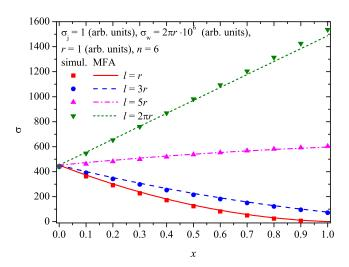
FIG. 8. Dependencies of the electrical conductance on the proportions of rings and sticks, x, for the fixed values of the number density of fillers and different values of l. MFA predictions are shown as curves, while markers correspond to the simulations. Here, r=1,  $R_{\rm j}=1$ , and  $\rho_{\rm w}=(2\pi r)^{-1}10^{-6}$ , n=6.
