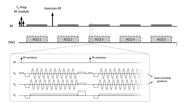
**Figure 1**: Pulse sequence diagram of the proposed wave-CAIPI 3D-QALAS sequence. The top of the figure shows one repetition period, where one can see the  $T_2$ -prep and inversion RF modules, as well as clearly distinguish the five echo-train readouts, each sampling covering the
