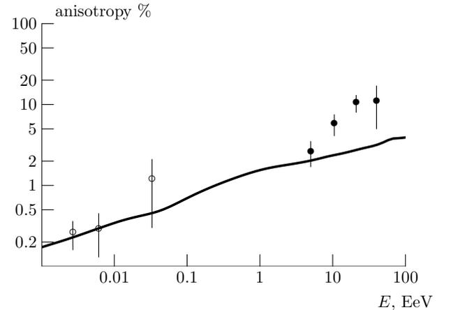
**Figure 4.** Calculated cosmic ray anisotropy (solid line). The results of Pierre Auger Collaboration (energy shift +10%, Aab et al. (2018) black circles) and KASCADE-Grande experiment (Chiavassa et al. (2015) open circles) are also shown.
