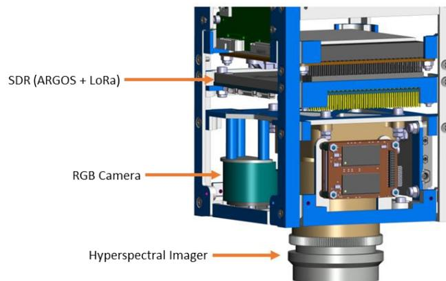
Figure 8. AEROS Spacecraft Payload Bay Arrangement. Credit: CEiiA
