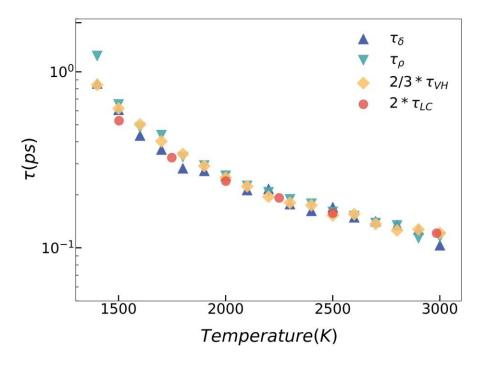
**Figure 8.** Temperature variation of the lifetime of  $C_{amp}(t)$ ,  $\tau_{\rho}$ , and  $C_{ph}(t)$ ,  $\tau_{\delta}$ , compared to  $2 \tau_{LC}$  and  $(2/3) \tau_{VH}$  for liquid Fe.
