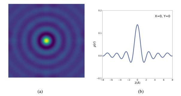
**Figure 9.** The  $\rho(\mathbf{r})$  centered at a single atom at  $\mathbf{r} = 0$  obtained by overlapping density waves with  $\delta_{IG} = 0$ . (a) 2D color map at z = 0, and (b) a cut at x = y = 0.
