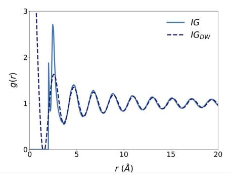
**Figure 5.** The PDF of the model of ideally coherent glass state for liquid Fe created by the RMC method (solid curve). The sharp peak at 2.0 Å reflects the imposed minimum atomic distance. The dashed curve represents eq. (29).
