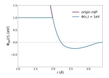
**Figure 2.** The modified Johnson potential (mJP) and  $\phi_{pp}(r)$  of Fe with  $\phi(r_c) = 1$  eV.
